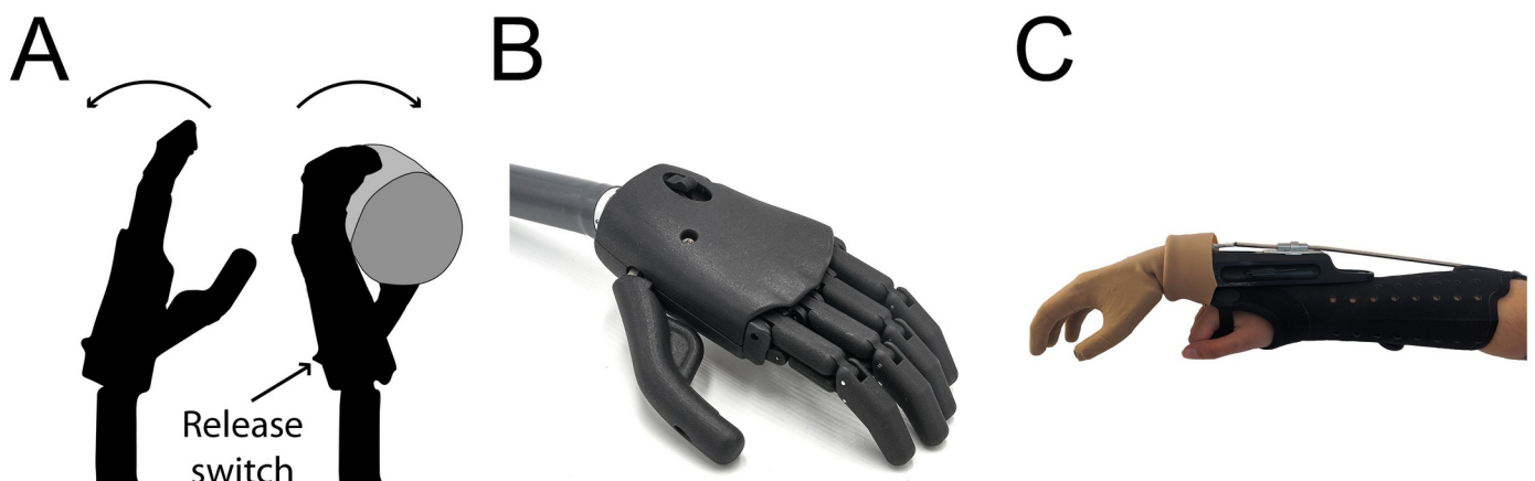
Fig 1. The Self-Grasping Hand. A: As the Self-Grasping Hand is flexed backward at the wrist, the fingers curl around the object. B: Self-Grasping Hand prototype. C: Self-Grasping Hand attached to the TRS simulator forearm brace with a cosmetic glove worn over the hand (Please note that the TRS simulator is designed for use with body-powered prostheses and therefore includes a cable running along the brace. This cable was not attached to the Self-Grasping Hand and was not used during this study).
