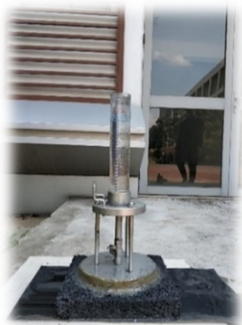
Fig.4. The permeability measurement device.
