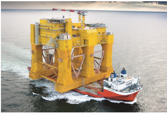
(a) Transport DolWin2 HVDC platform
