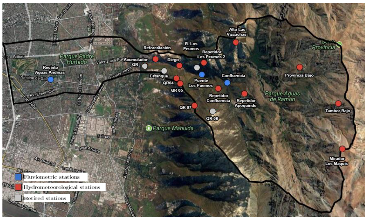
Fig. 1. Map of the Quebrada de Ramón wireless sensor network for early warning of flash floods.
