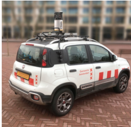
Figure 5.1.: The car of the City of Amsterdam that is used to capture SVI from Amsterdam, equipped with a 360° Tribble MX7 mobile imaging system. Source: [Geospatial, 2022]
