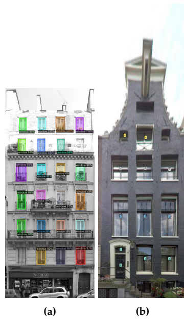
Figure 6.11.: The general undershooting of the floor count determination method is often due to non-detection of smaller windows or unknown class shop.
