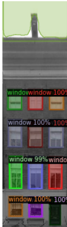
Figure 1.2.: Façade parsing example: identification and segmentation of windows and doors. The aim in this thesis is to count the number of storeys from the repetitive occurrence of windows and doors.
