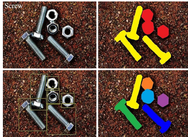
Figure 2.13.: Different types of computer vision tasks, from coarse to finer-grained. Top row: classification and semantic segmentation. Bottom row: object detection and instance segmentation. Adapted from Sharma et al. [2022].
