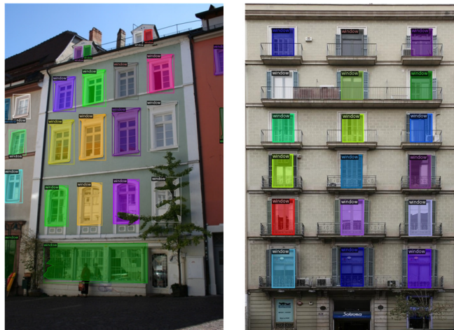
Figure 2.25.: Façade parsing results of DeepWindows [Sun et al., 2022]. A limiting factor for the determination of floor count would be the lack of door detection. In a few cases, the ground floor has a door but no windows.
