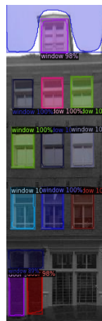
Figure 4.7.: For this particular façade, the point selection matters for the outcome of the floor count determination. Note the smaller windows above the doors (bottom left).
