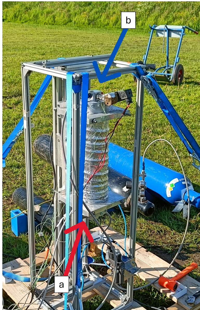
Figure 3.16: Image of the run-tank. The red arrow (bottom, labelled (a)) indicates the extraction from the bottom of the tank, the blue arrow (top, labelled (b)) shows the new location for the third test.
