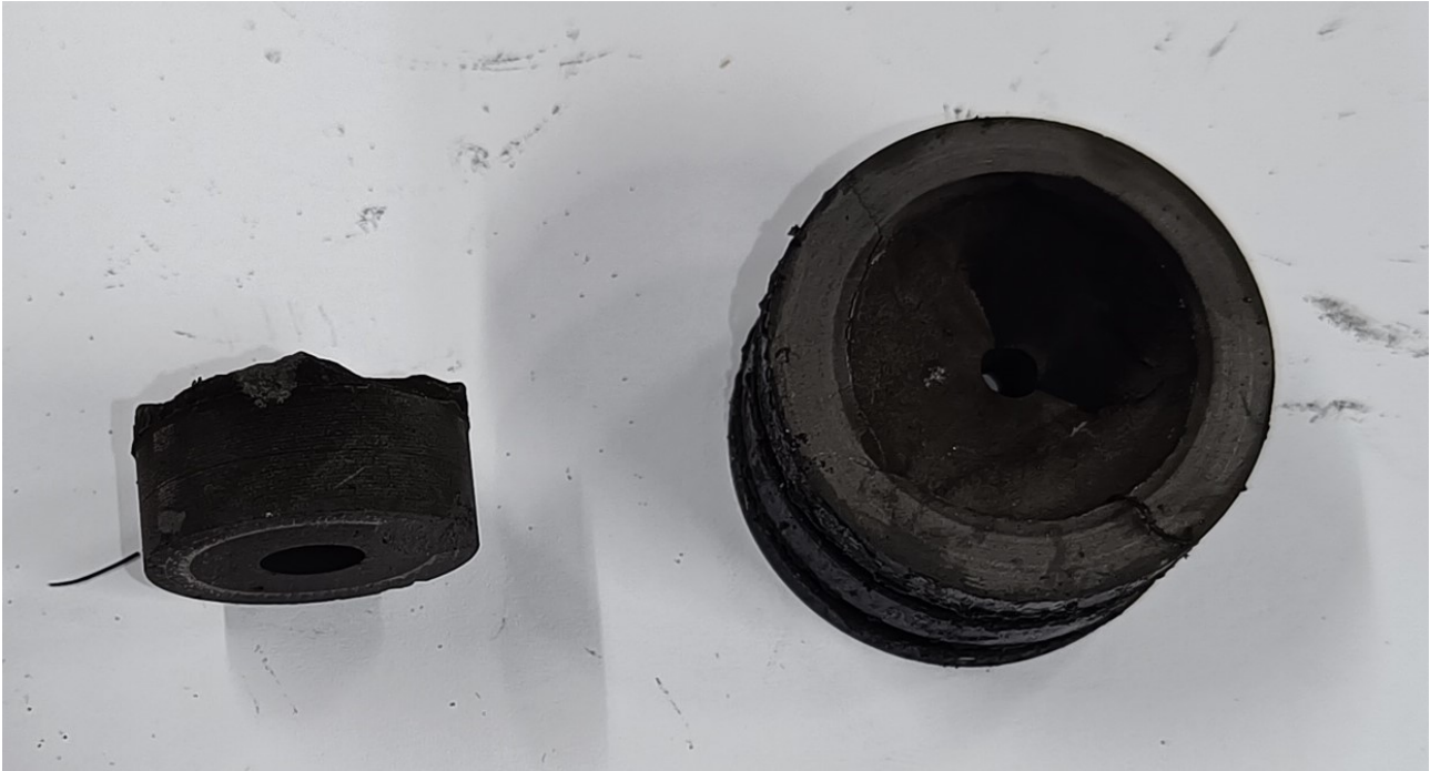
Figure 3.14: Broken graphite nozzle from double hole test 2.
