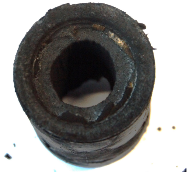
(b) Reference grain (test 1) after test.
