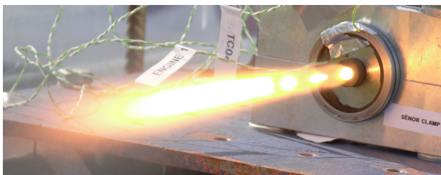
(a) Double anchor grain at start of engine test.
