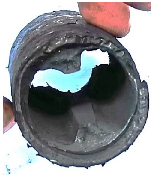
(b) Double anchor grain (test 3) after test.
