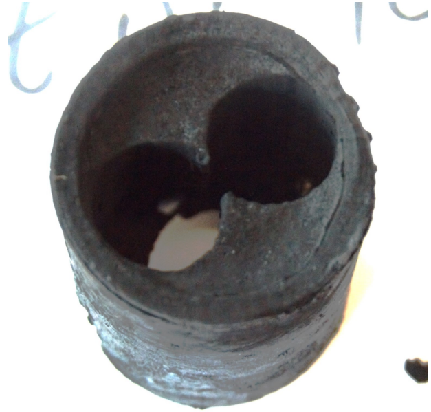
(b) Double hole geometry after first test.
