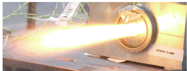
(b) Double anchor grain after nozzle broke.
