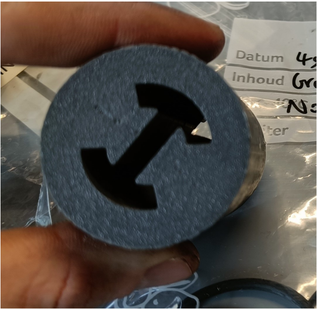
(a) Double anchor geometry before first test.
