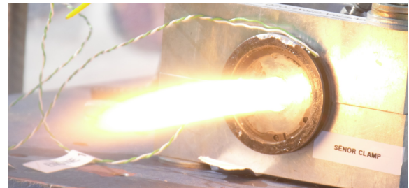
(b) Reference grain after nozzle broke.
