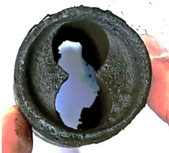
(b) Double hole grain (test 3) after test.
