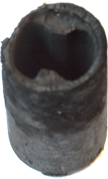
(b) Double anchor geometry after first test.
