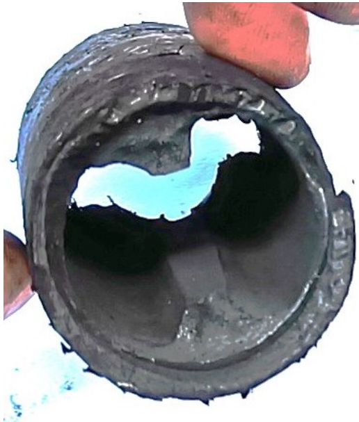
(b) Double anchor geometry after third test.
