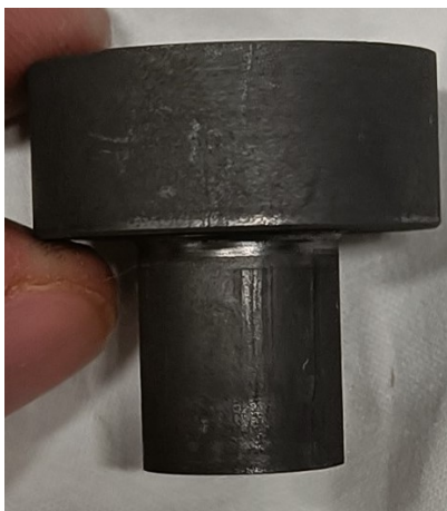
(a) Nominal version 1 of the graphite nozzle.
