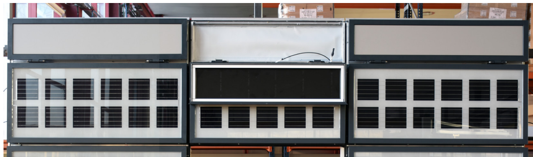
FIG. 13 Full-scale prototype, combining RIVENTI's and ONYX's technologies. 3 access zones can be seen at the top of the sample. The central access zone is opened, and the lateral ones are closed.
