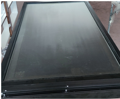
FIG. 8 Prototype of ST panel combining RIVENTI's and KAMEL's technologies.
