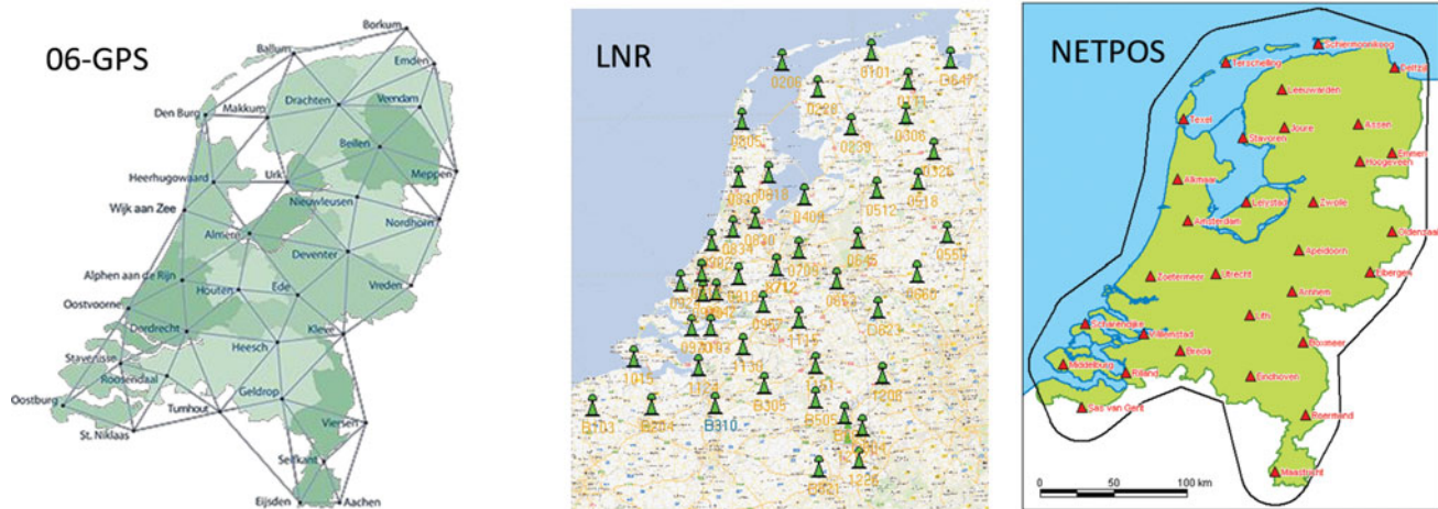
Fig. 14. RTK Networks in the Netherlands, with on the left the 06-GPS network, in the middle LNR-GlobalCom network, and on the right the NETPOS network.
