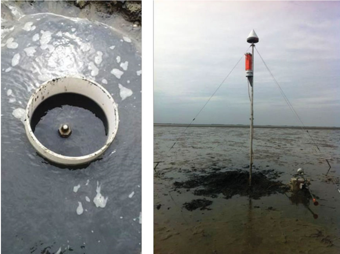
Fig. 28. Typical GPS benchmark (left) and GPS measurement set-up (right) in the Wadden Sea area (pictures courtesy NAM).
