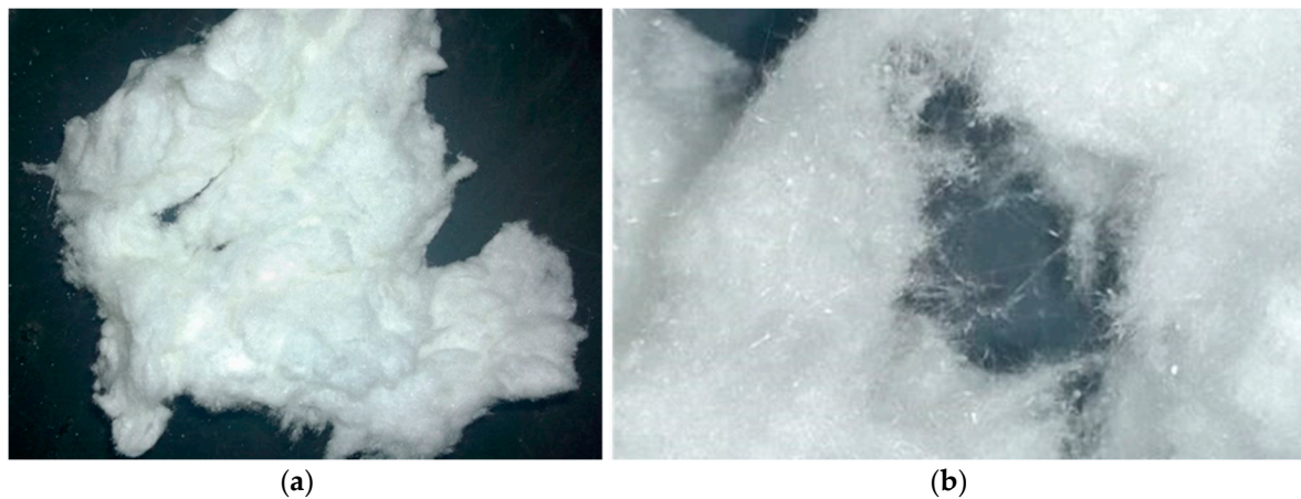
Figure 1. Ceramic fiber used in this research ((a) cluster view; (b) closer view).
