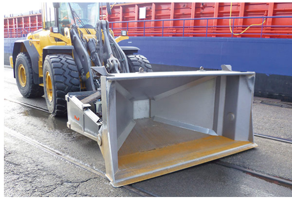
Figure 4.23: A hopper bin, i.e. an example for a water collection funnel (Verachtert Nederland B.V, 2024)
