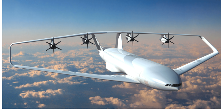
Figure 1.2: An example of a box wing aircraft. [5]
