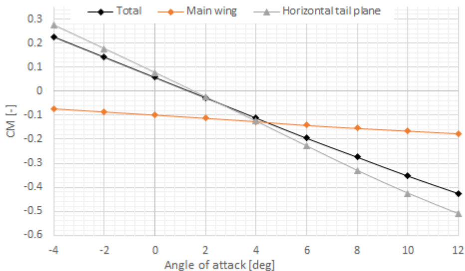
Figure 4.13: Calculated contribution by VSAero of the main wing and horizontal tail plane to the moment curve C_m versus \alpha for the CRM.
