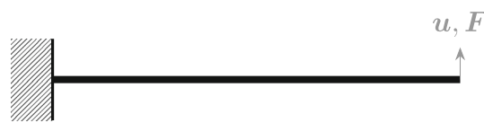
Fig. 2 Schematic of a cantilever beam under load
