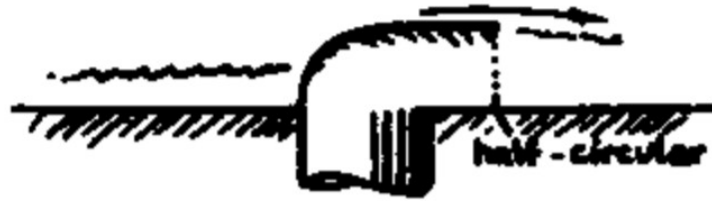
Figure 7.16: Geometry of the outlet for the propulsion system. The inlet is not raised from the surface in order to minimise drag and since boundary layer concerns do not apply here.
