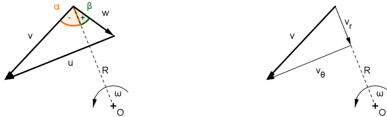
(a) Components in the absolute and relative frame of reference (b) Components of one vector in the the frame of reference (r, \theta)
