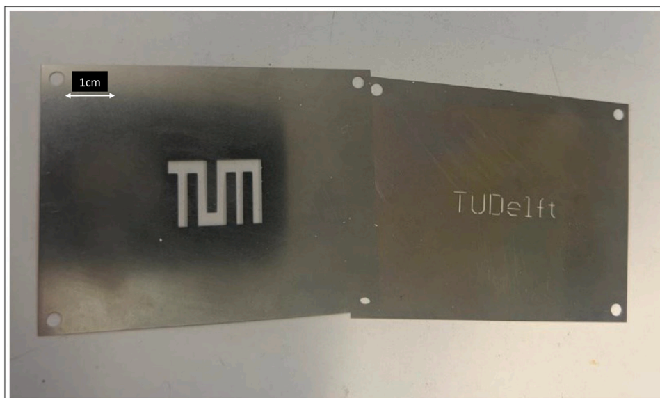
Fig. 4. 100 \mu\text{m} thick masks with different patterns. The TUM and TUDelft logo masks are used to create patterns on both sides of a Mylar foil sample.
