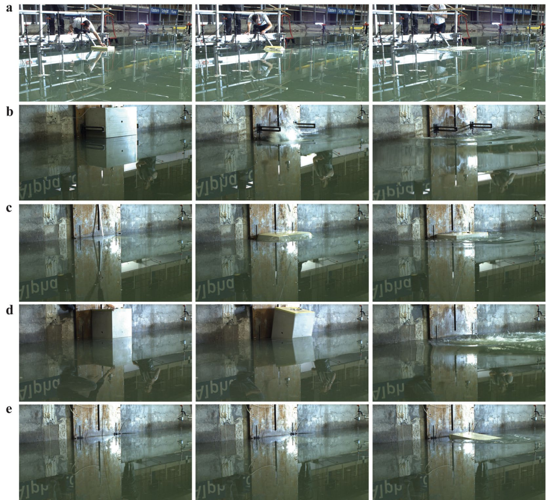
Figure 2. Image series of our large-scale experiments conducted in the basin at a water depth of 1.00 m. (a) Capsizing (mechanism A). (b) Gravity-dominated fall (B). (c) Buoyancy-dominated fall (C). (d) Gravity-dominated overturning (D). (e) Buoyancy-dominated overturning (E). The shown examples of mechanisms A and E were conducted with a 0.800 m × 0.500 m × 0.250 m block (type 2) and the two examples of mechanisms B, C and D with a 0.800 m × 0.500 m × 0.500 m block (type 1). Wave profiles and movies for the five mechanisms are shown in Fig. 4 and the Supplementary Information.
