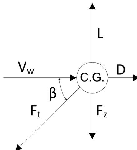
Figure 2.8: The free body diagram for a kite which is considered to be a point mass.
