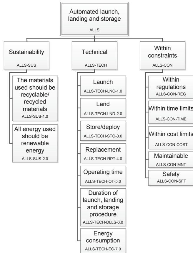
Figure 2.1: Top-level requirements for the launch, landing and storage system
