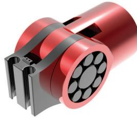
Figure 6.2: Detailed drawing of the beam hinge mechanism
