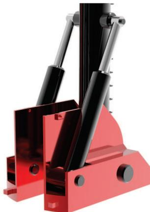
Figure 7.2: Detailed drawing of the boom hinge mechanism
