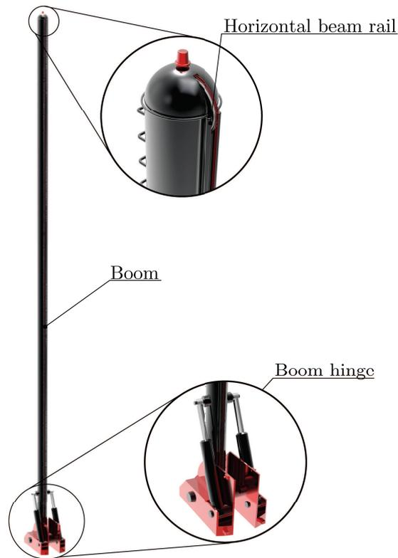
Figure 2.20: Overview of mechanisms within the vertical boom subsystem
