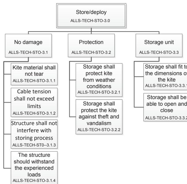
Figure 2.4: Low-level requirements for the storage/deployment procedure
