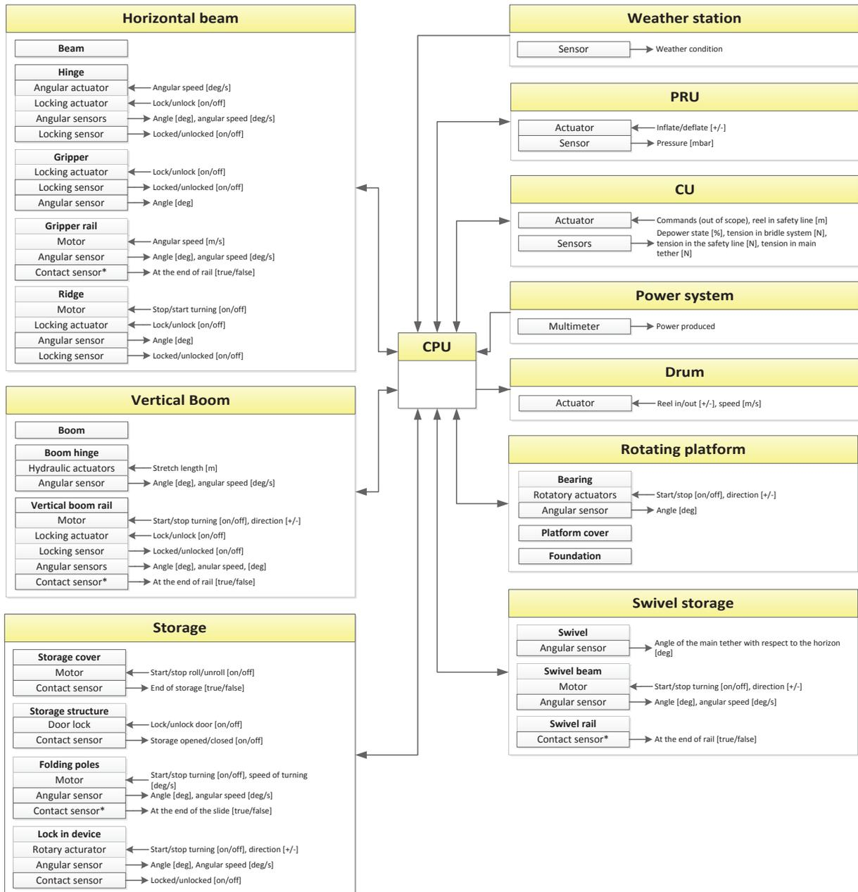
Figure F.1: Communication flow and data handling diagram
