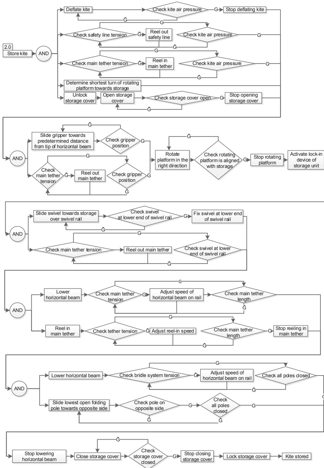
Figure A.2: Low-level functional flow diagram of the storage procedure
