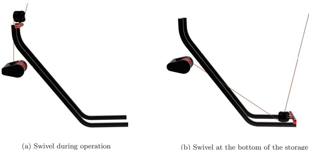
Figure 9.1: Detailed drawing of the swivel mechanism
