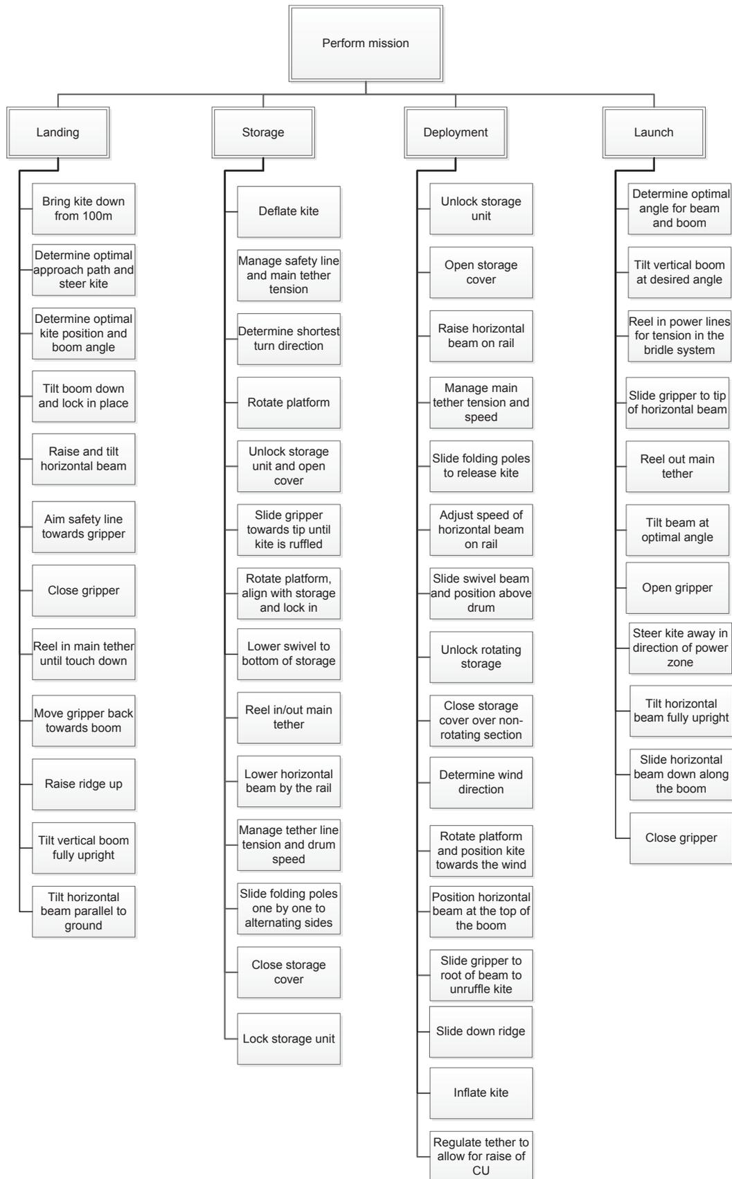
Figure A.5: Functional breakdown structure of the complete system
