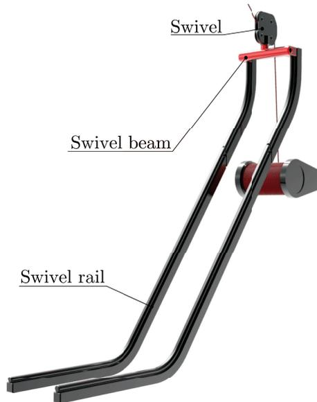
Figure 2.22: Overview of mechanisms within the swivel storage subsystem
