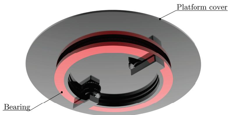
Figure 2.21: Overview of mechanisms within the rotating platform subsystem, seen from below
