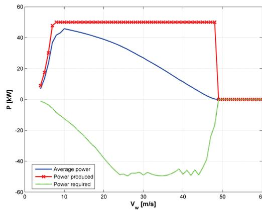
Figure 2.12: The power curve of a 50kW 70m<sup>2</sup> kite system.
