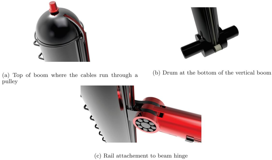
Figure 7.3: Detailed drawing of the vertical boom rail mechanism
