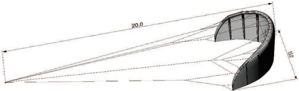
Figure 2.5: The overall dimensions of the kite in meters
