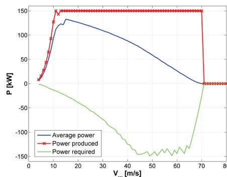
Figure 12.4: Power curve of a  $150kW$  system using the same kite and tether
