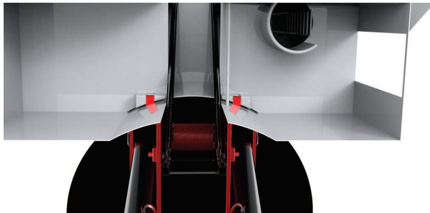
Figure 10.4: Top view detailed drawing of the lock-in device mechanism
