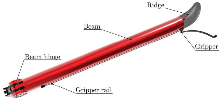
Figure 2.19: Overview of mechanisms within the horizontal beam subsystem
