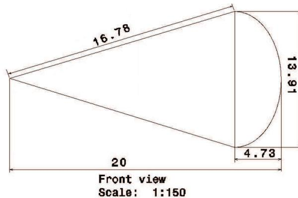
Figure 2.6: The detailed dimensions of the kite in meters
