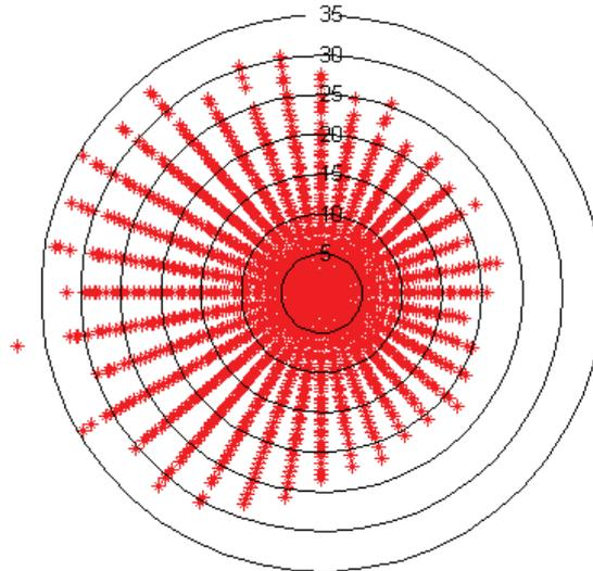
Figure 3.5: The wind distribution at Valkenburg from 1951 onwards, corrected for  $35m$  height
