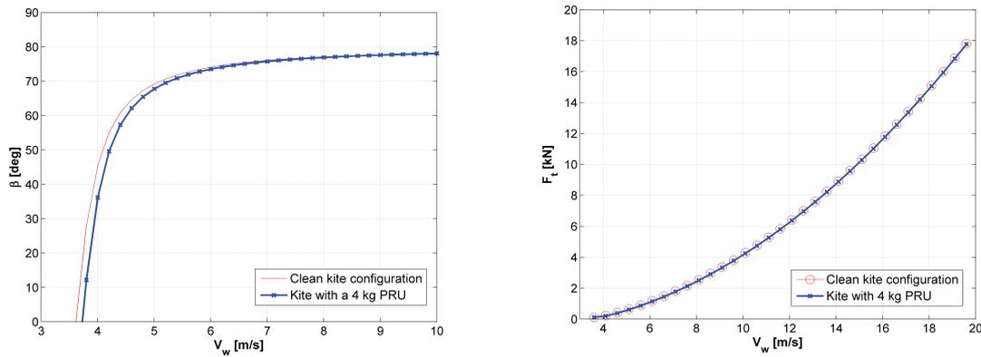
(a) The maximum tether angle  $\beta$  for different wind speeds (b) The tether force  $F_t$  for different wind speeds
