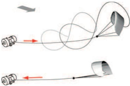
Figure 2.10: Overview of the pumping cycle
