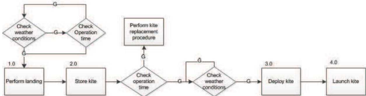
Figure 2.24: Top-level functional flow diagram
