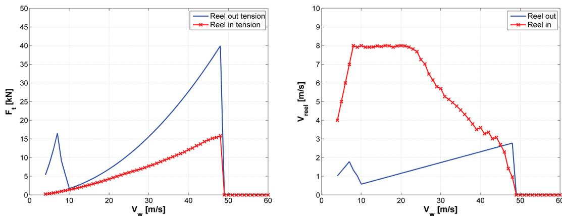
(a) The tether force  $F_t$  during reel out phase      (b) The reeling speeds for reeling out and reeling in
