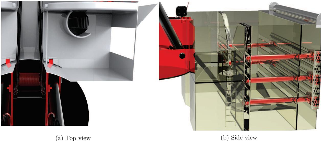
Figure 11.7: Access door and stairs in the storage unit for maintenance
