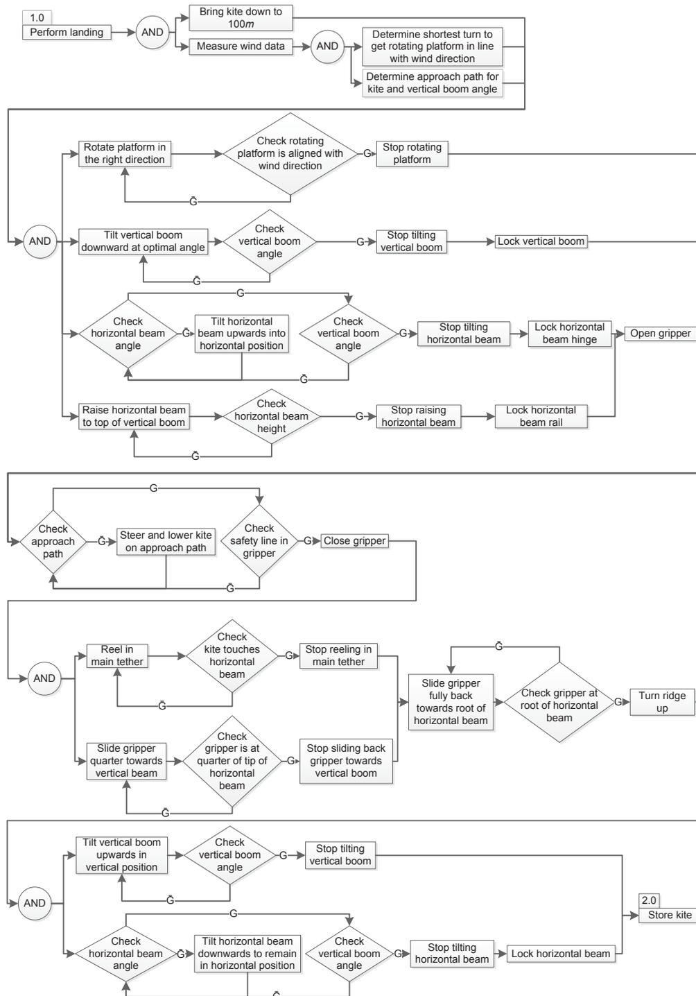
Figure A.1: Low-level functional flow diagram of the landing procedure
