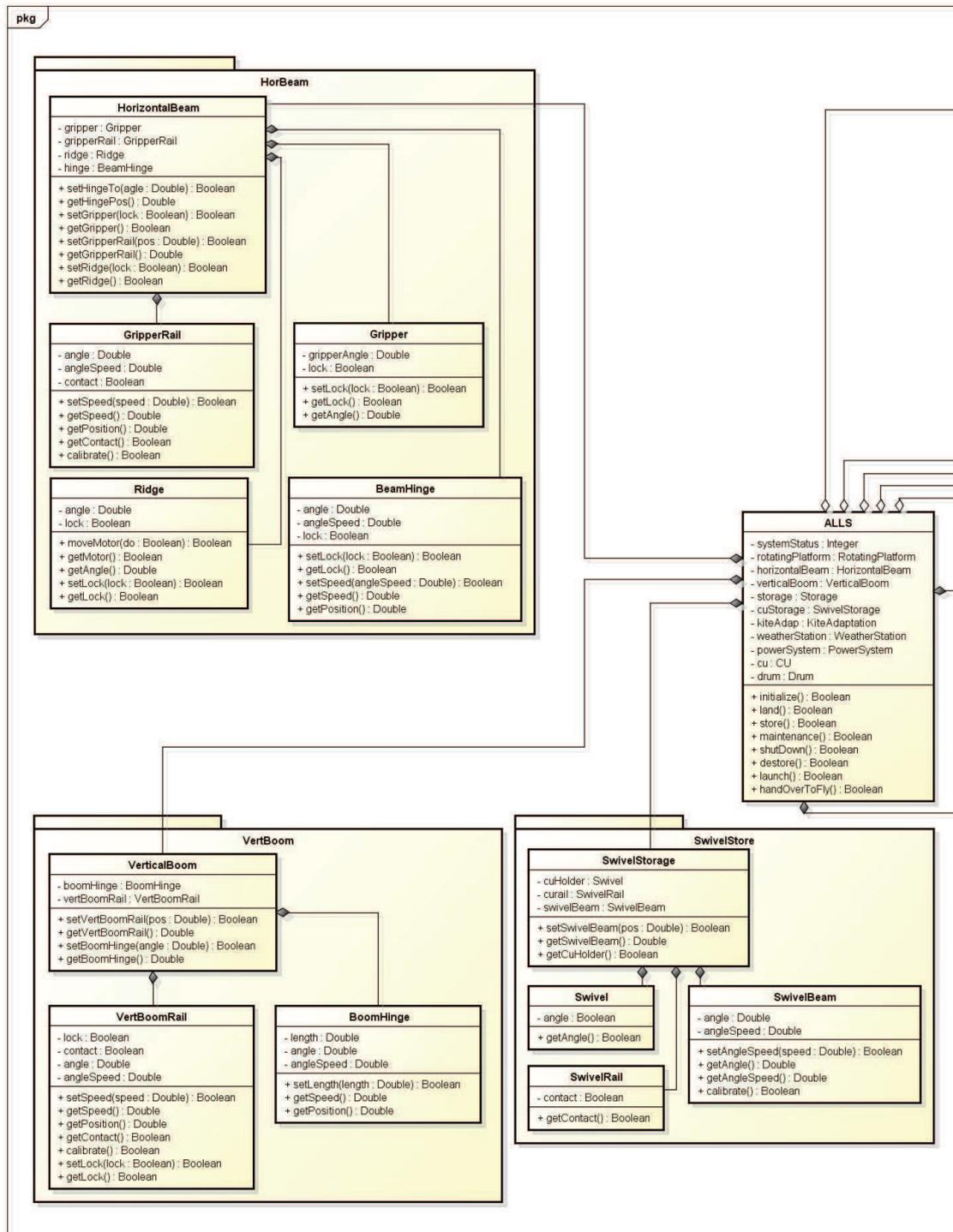
Figure G.1: Software (class) diagram (left part)
