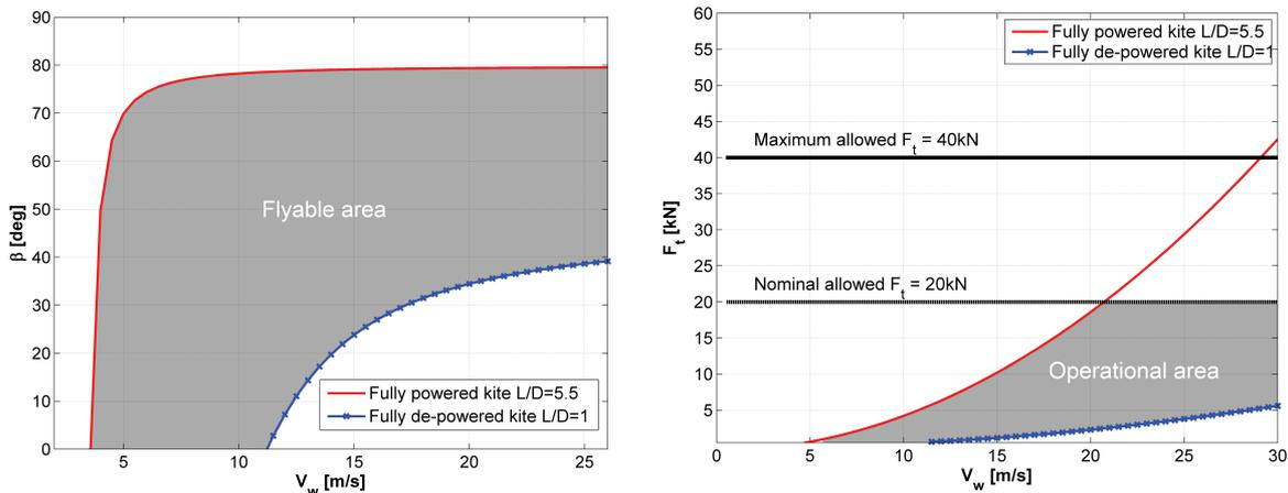
(a) The angle between the tether and the wind vector for different wind speeds
