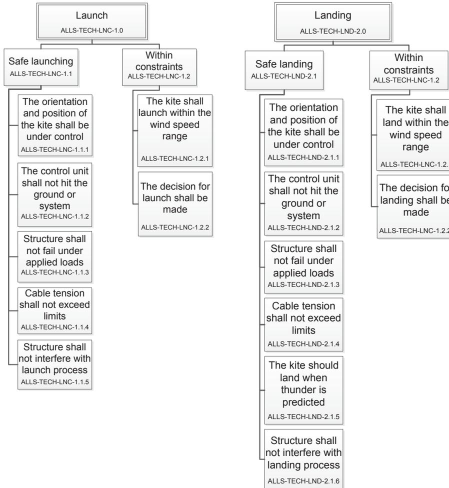
Figure 2.2: Low-level requirements for the launch procedure
