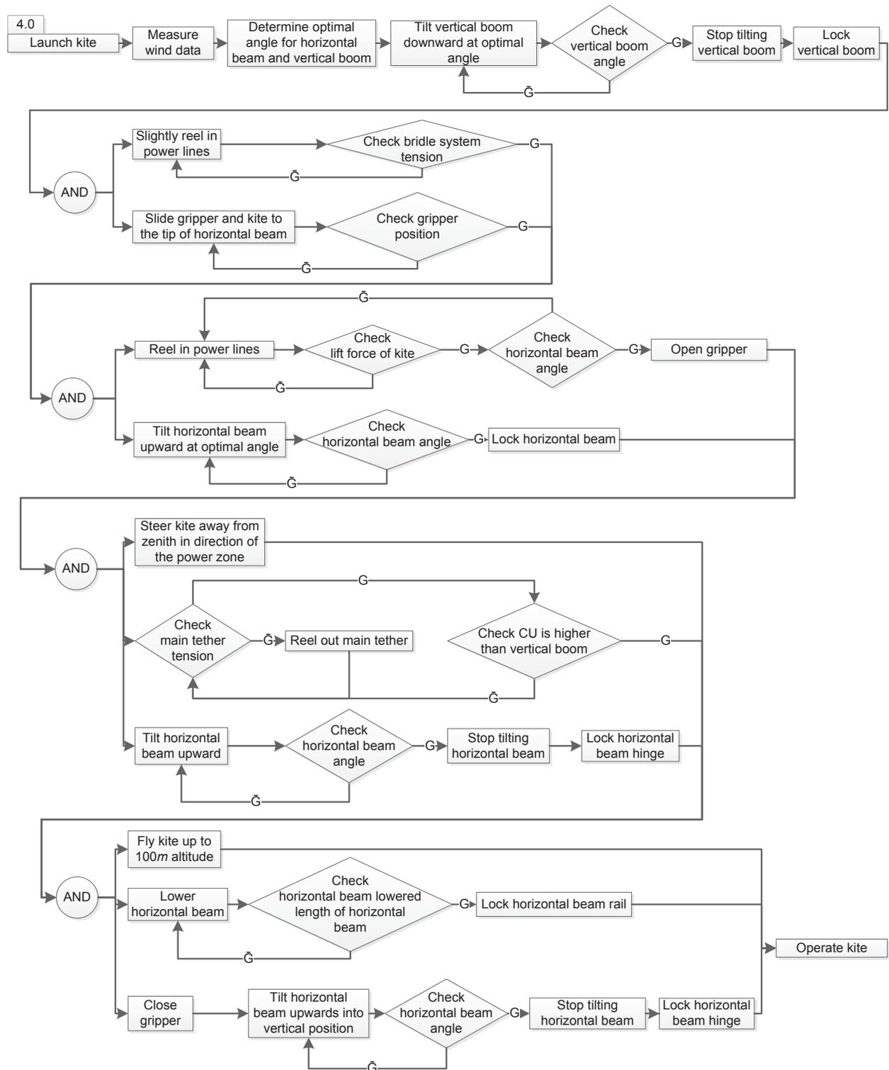
Figure A.4: Low-level functional flow diagram of the launch procedure
