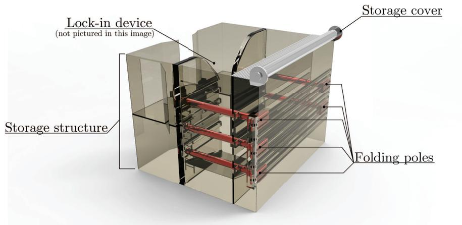
Figure 2.23: Overview of mechanisms within the storage subsystem
