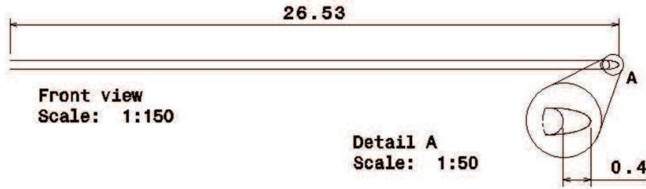
Figure 2.7: The detailed dimensions of the folded kite in meters
