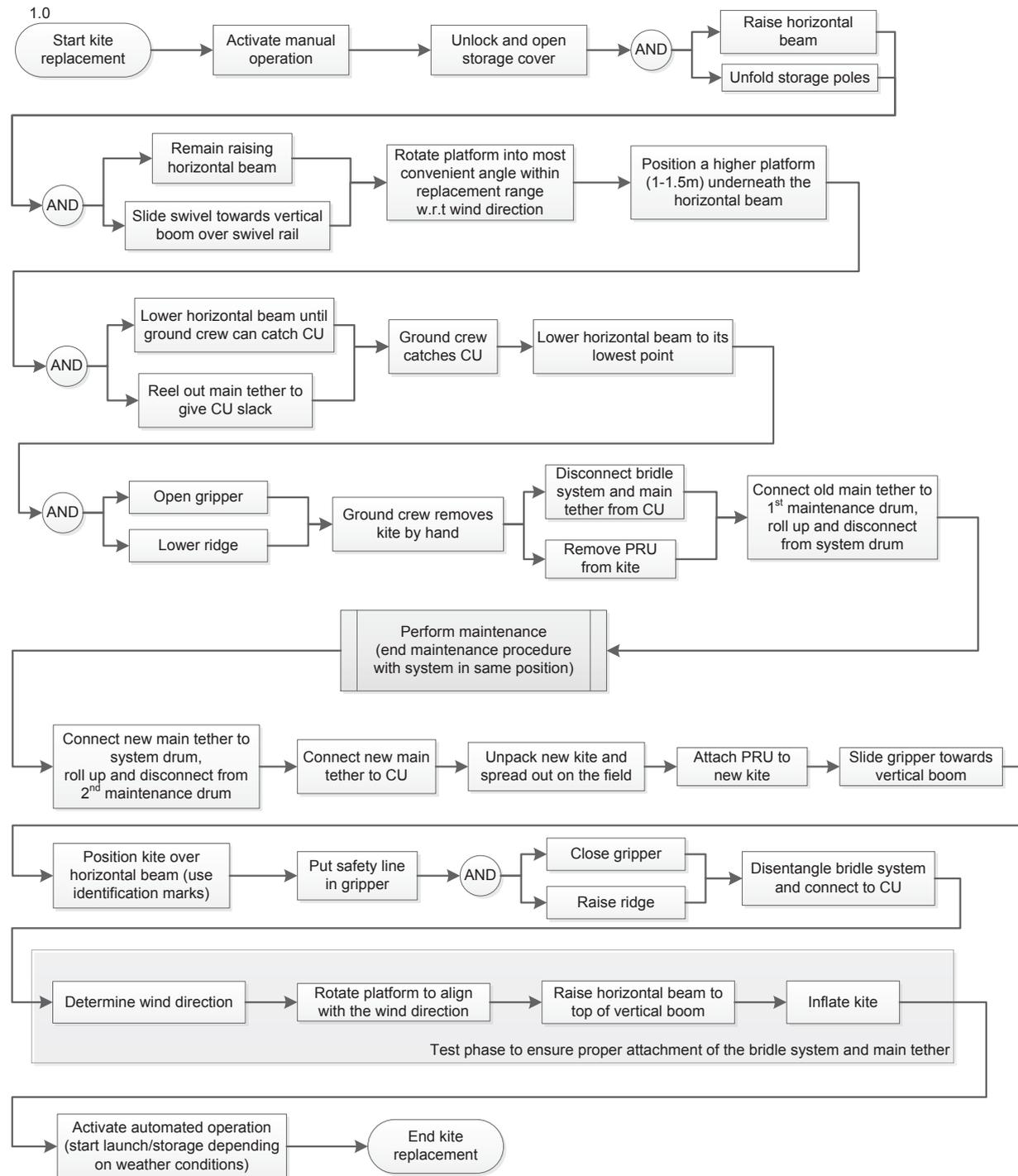
Figure C.1: Kite replacement procedure
