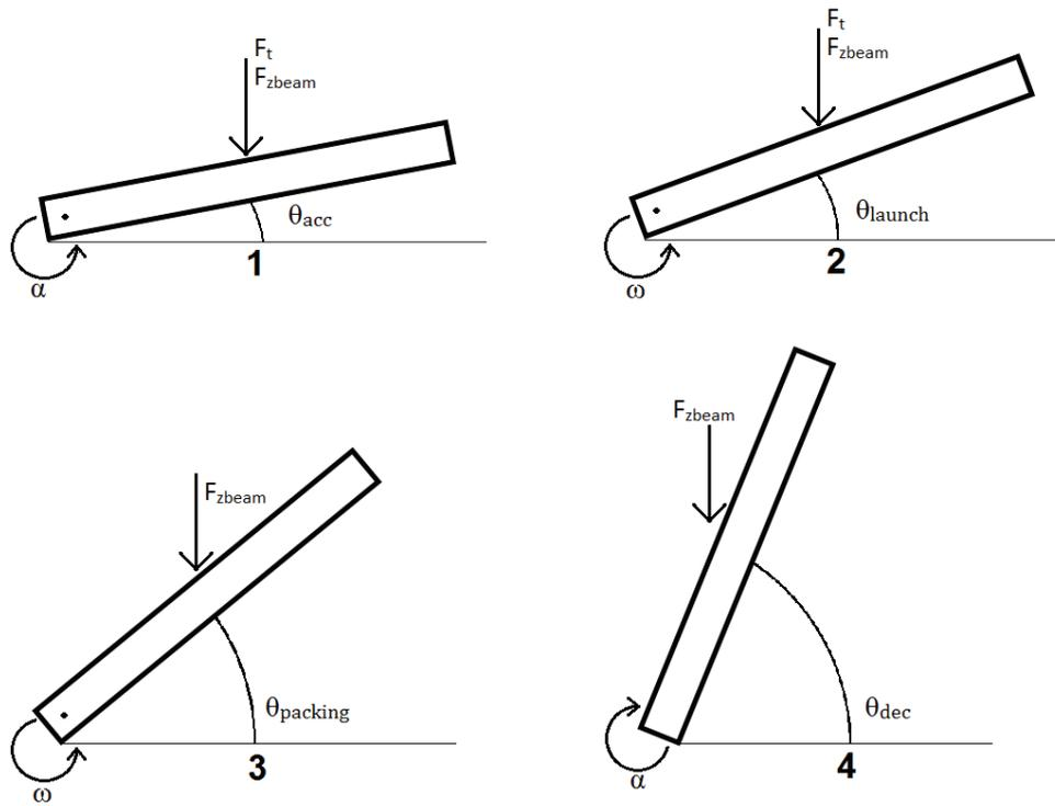
Figure 4.3: the four respective phases required for the *Horizontal Beam Hinge for Launch* energy calculation
