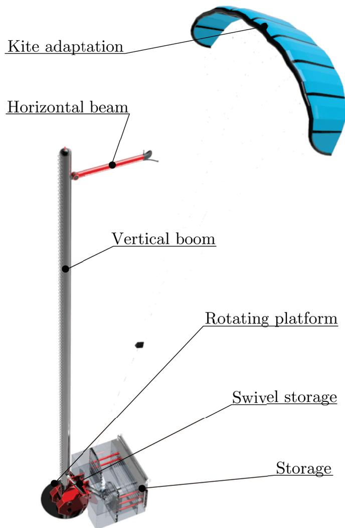
Figure 2.14: Overview of the automated launch, landing and storage system with all subsystems
