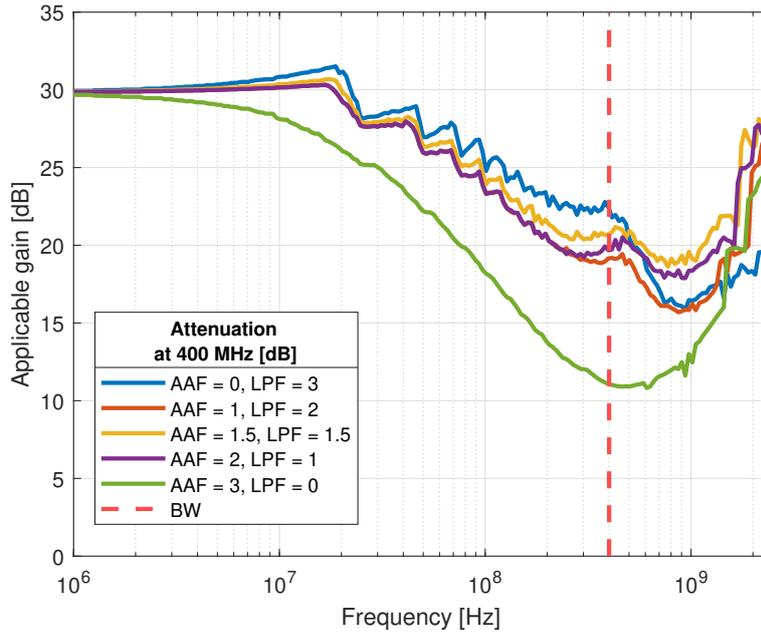
Figure 4.15: Applicable gain versus frequency, for a 4<sup>th</sup> order APF
