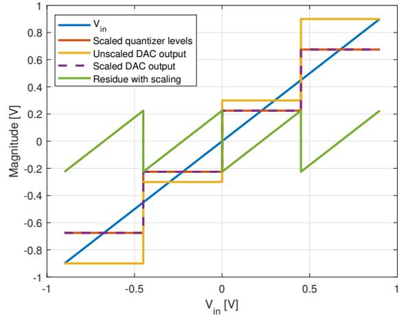
Figure 4.21: Scaled quantizer levels and DAC, with the residue signal
