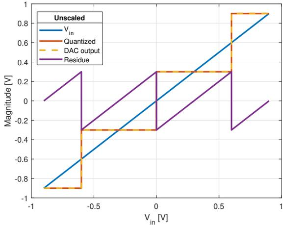
Figure 4.20: Unscaled quantizer levels and DAC, with the residue signal
