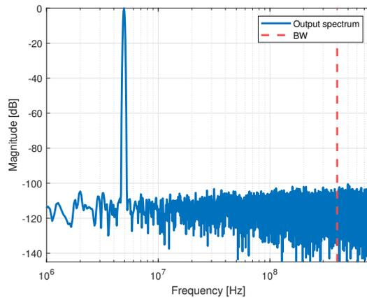
Figure 5.17: Output spectrum MATLAB®,  $f_{in} = 5$  MHz
