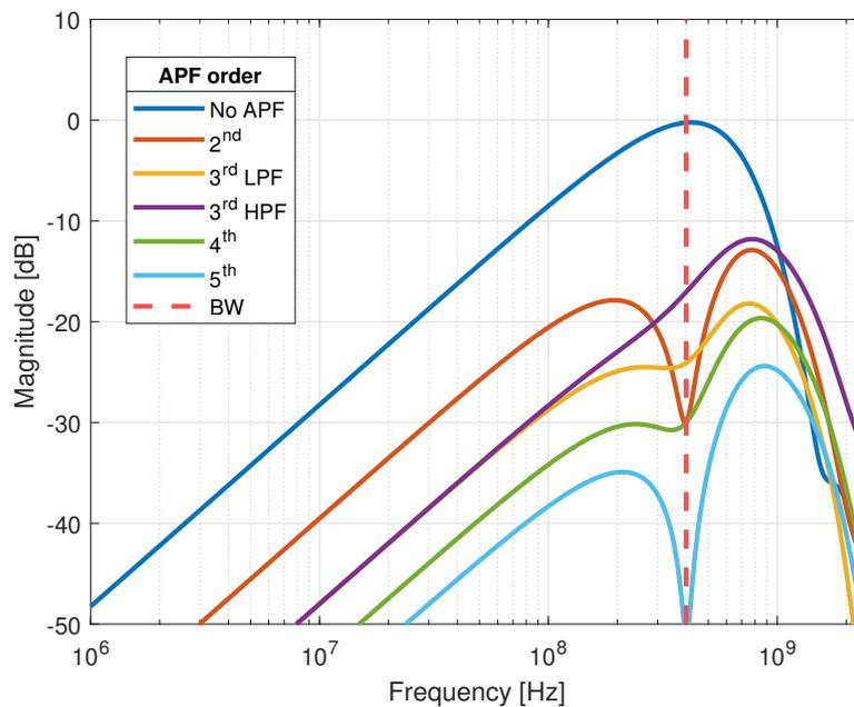
**Figure 4.11:** Magnitude of residue signal, with all (AAF, LPF and the APFs) the filters implemented
