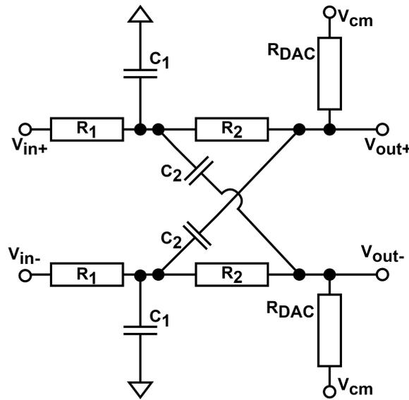
**Figure 6.10:** APF for the open loop implementation, with the added shunted capacitor
