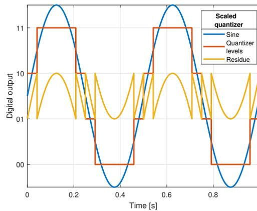
Figure 4.19: Scaled 2 bit quantizer
