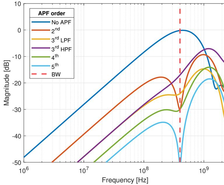
**Figure 4.10:** Magnitude of residue signal, with a LPF and the APFs implemented
