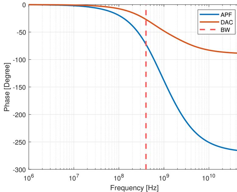
**Figure 6.14:** Phase response of the APF and DAC, combined with the first LPF for the open loop implementation
