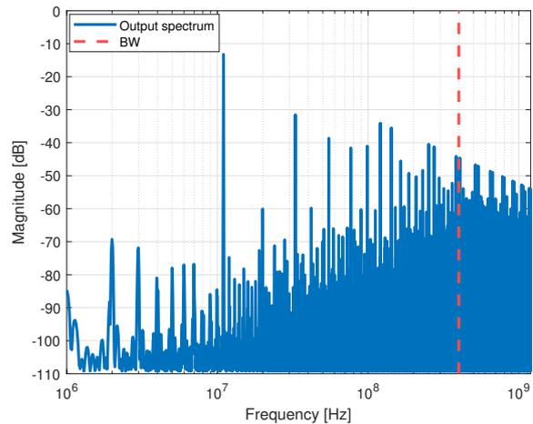
Figure 4.23: Scaled ADC & DAC spectrum,  $f_{in}=11\text{MHz}$
