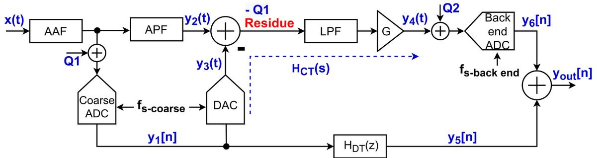
Figure 3.1: Block diagram of the two-stage system architecture
