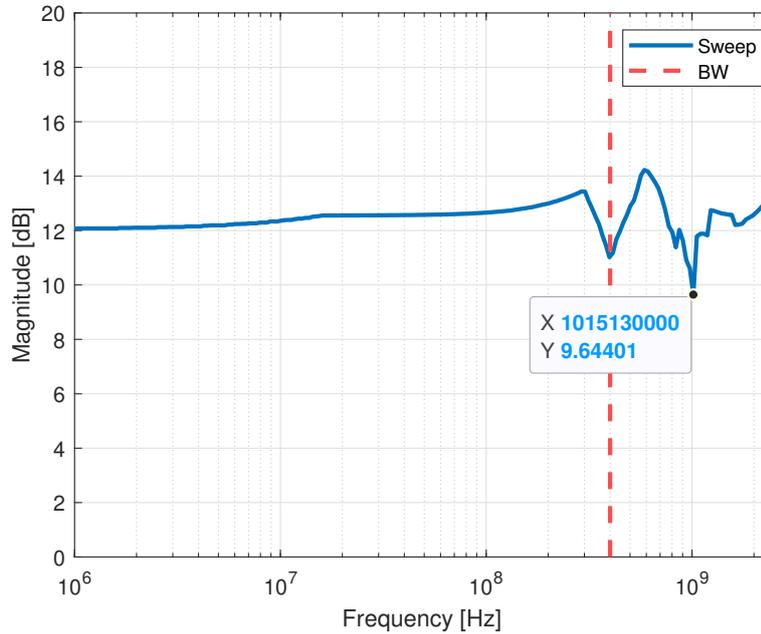
**Figure 5.13:** The applicable gain after the LPF versus frequency for the first-stage, for a 2<sup>nd</sup> order APF
