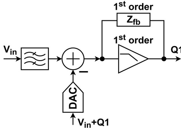
Figure 6.21: Closed loop 2<sup>nd</sup> order LPF realization
