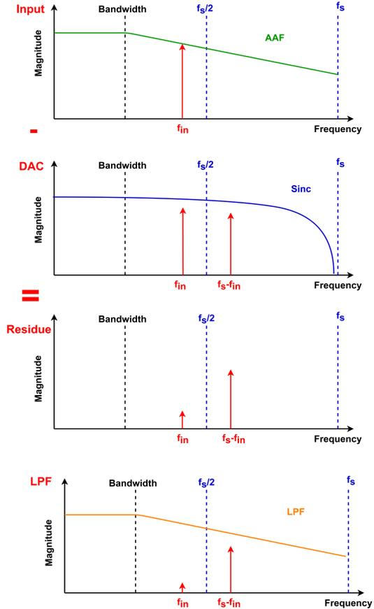
Figure 4.2: Attenuation of an OOB interferer
