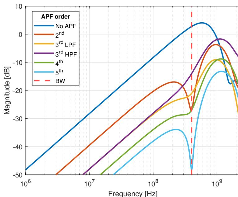
**Figure 4.9:** Magnitude of residue signal, with an AAF and the APFs implemented
