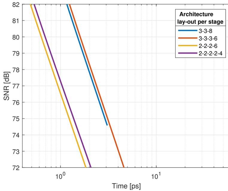
**Figure 5.6:** Time mismatch for the architectures
