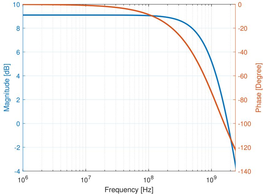
**Figure 6.1:** Transfer function of the required LPF, 0.75dB at 400MHz
