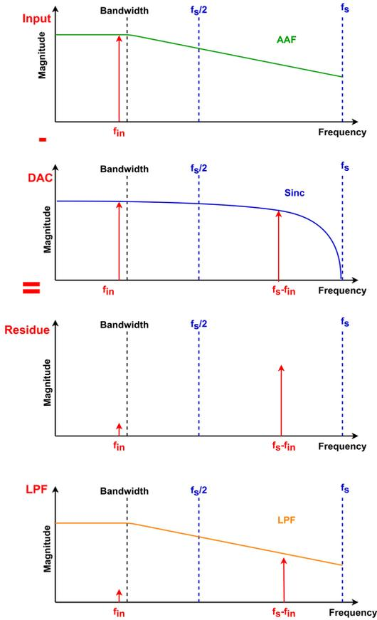
Figure 4.1: Attenuation of an in-band signal
