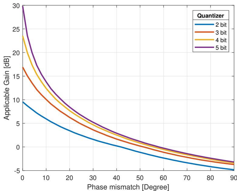
**Figure 4.17:** Applicable gain versus phase mismatch between the DAC and APF output, for different amount of resolved bits, with an ideal latency compensation and equal sampling rates
