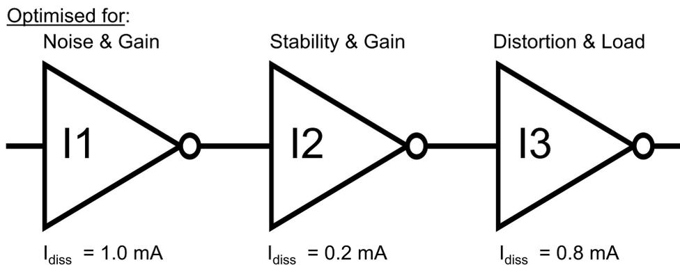
**Figure 6.22:** Inverter budget closed loop amplifier
