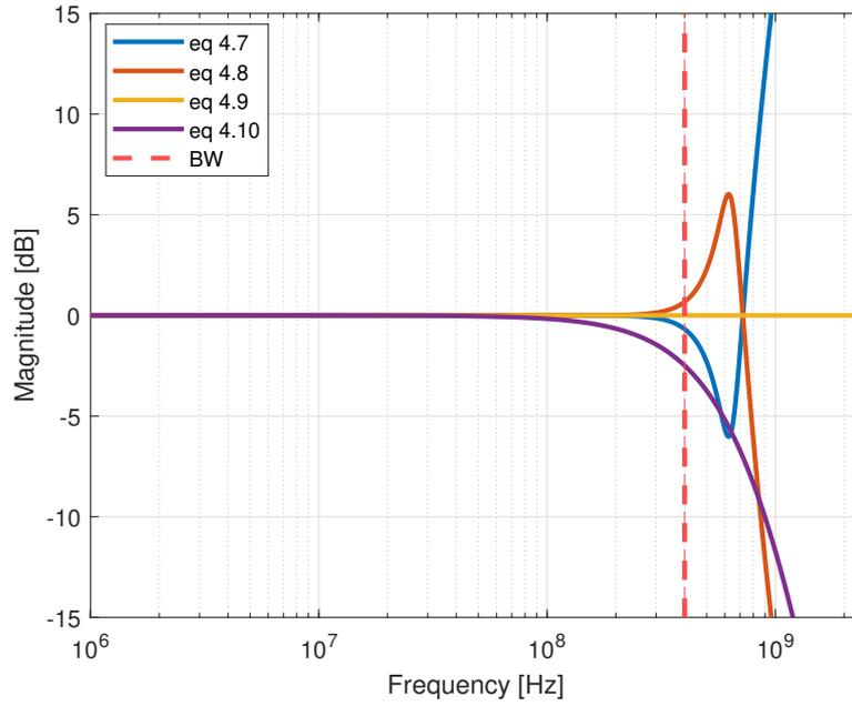
Figure 4.7: Magnitude response of the 4<sup>th</sup> order transfer functions,  $\tau = \frac{1.5}{f_s}$
