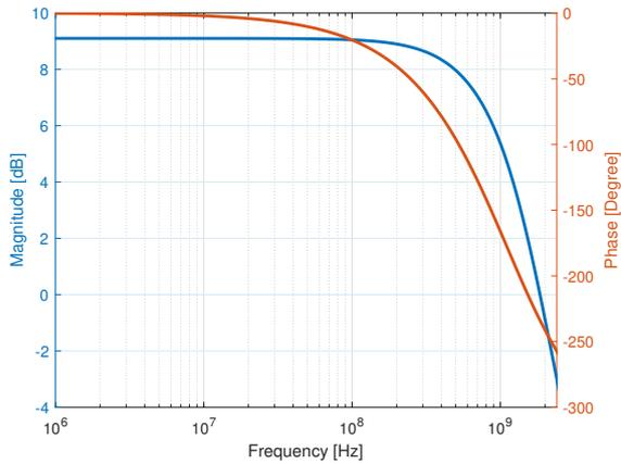
Figure 6.24: Transfer function closed loop amplifier
