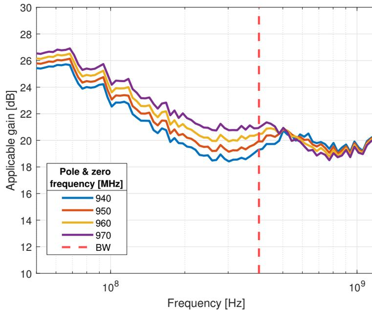
**Figure 4.12:** Applicable gain after LPF, for different latencies of the 4<sup>th</sup> order APF
