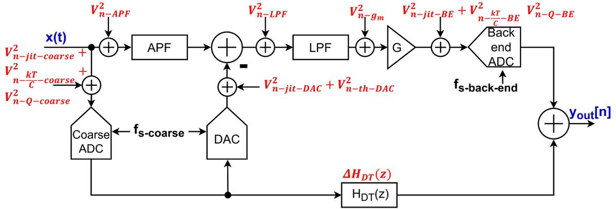
Figure 5.1: The main noise sources for a two-stage architecture
