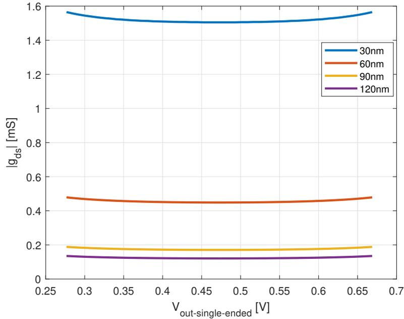
**Figure 6.19:** The output resistance versus the single ended output swing
