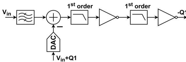
**Figure 6.4:** Open loop LPF implementation, with two cascaded LPFs
