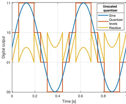
Figure 4.18: Unscaled 2 bit quantizer
