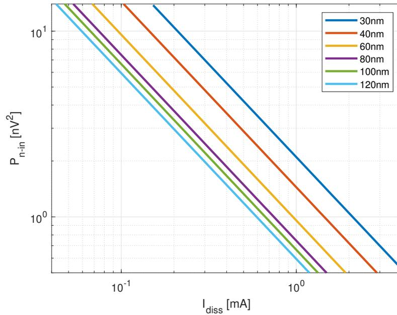
**Figure 6.16:** Input referred integrated noise voltage versus current dissipation, for different transistor lengths of the inverter
