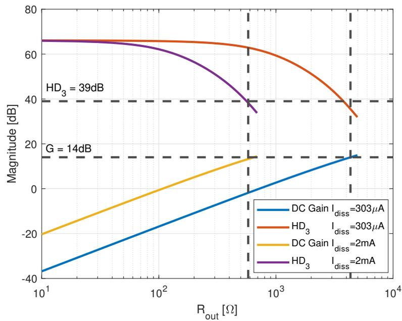
**Figure 6.18:**  $HD_3$  versus resistance of the LPF, for different currents, for a length of 120nm
