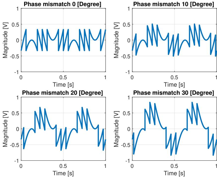
Figure 3.2: Residue output due to phase mismatch
