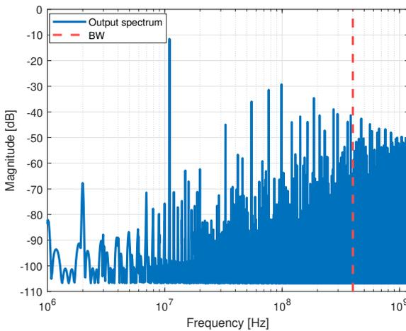
Figure 4.22: Unscaled ADC & DAC spectrum,  $f_{in}=11\text{MHz}$
