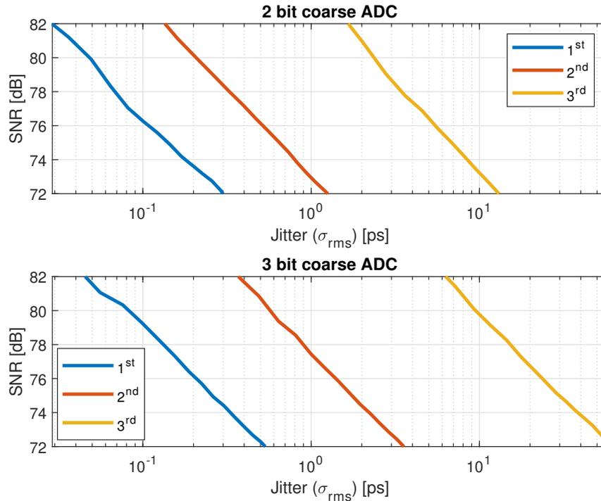
**Figure 5.3:** DAC jitter of the four-stage architecture, 2 bit versus 3 bit coarse ADC for the different stages
