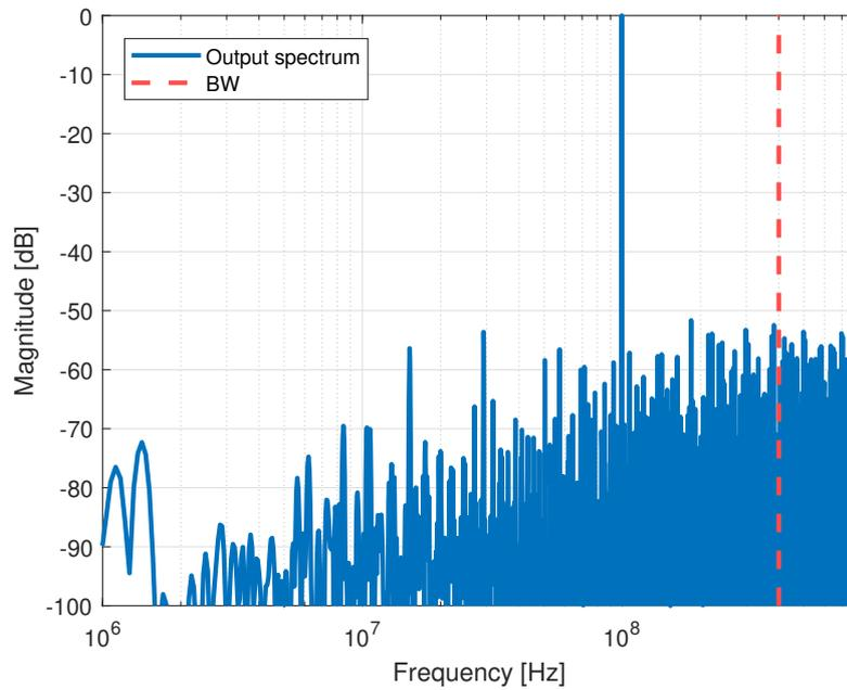
**Figure 5.12:** Output spectrum of the back end ADC for a full scale input signal
