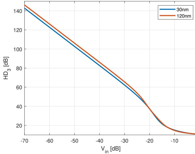
**Figure 6.17:**  $HD_3$  versus  $V_{in}$  for transistor lengths of 30nm and 120nm, for the same current
