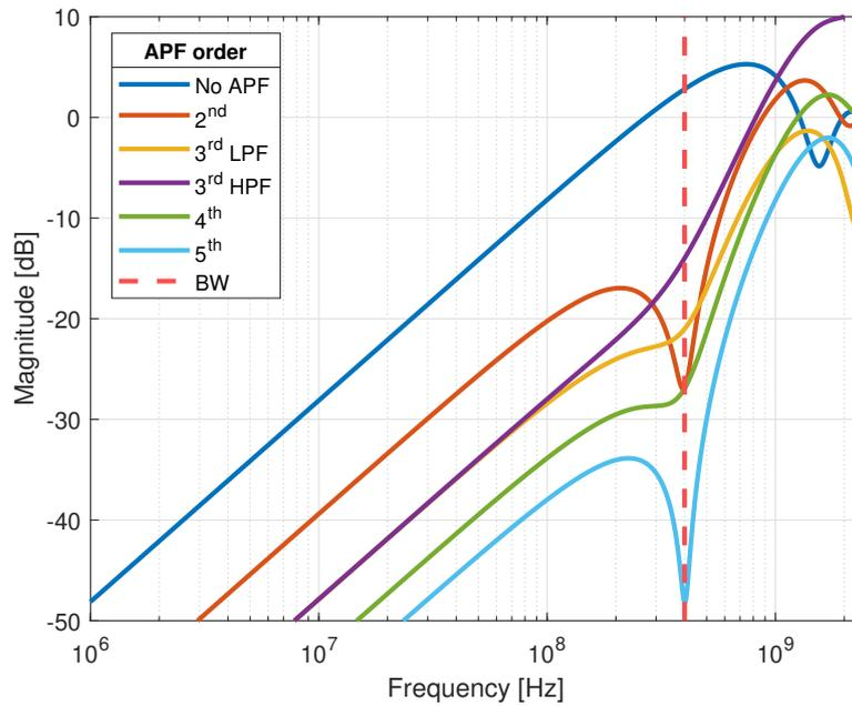
**Figure 4.8:** Magnitude of residue signal, with only the APFs implemented
