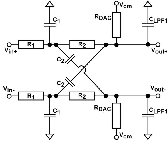
Figure 6.11: APF for the open loop implementation, with the LPF added
