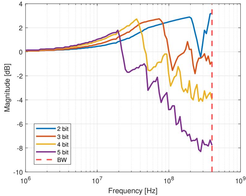
**Figure 4.14:** Gain after LPF, for different amount of bits, for an 4<sup>th</sup> order APF, latency of 625ps and the LPF has 3dB attenuation at 400MHz ( $f_{-3dB}=622\text{MHz}$ ). Note that for a better visualization of the LPF impact, the DC gains are normalized to 0dB
