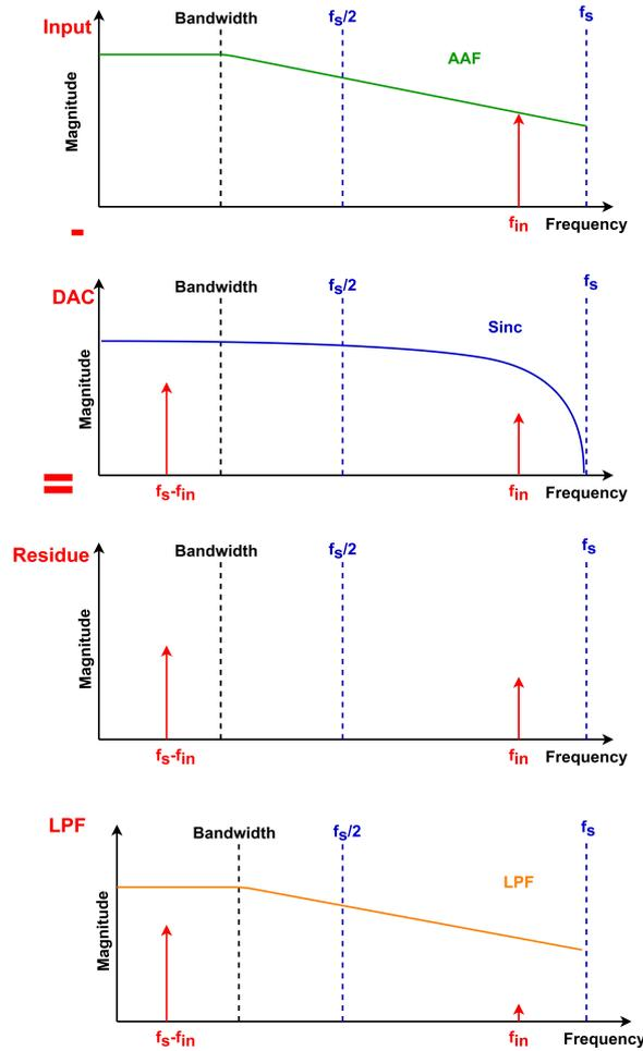
Figure 4.3: Attenuation of a far OOB interferer
