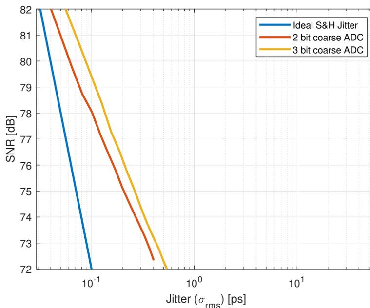
**Figure 5.2:** DAC jitter for the 2 bit versus 3 bit coarse ADC
