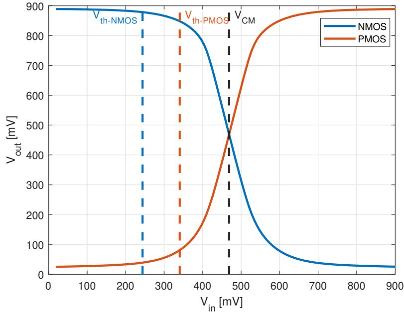
**Figure 6.15:** Operation region inverter, for a gain of 14dB and gate length = 30nm
