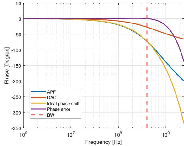
**Figure 6.13:** Phase response of the APF and DAC for the open loop implementation, with the phase error
