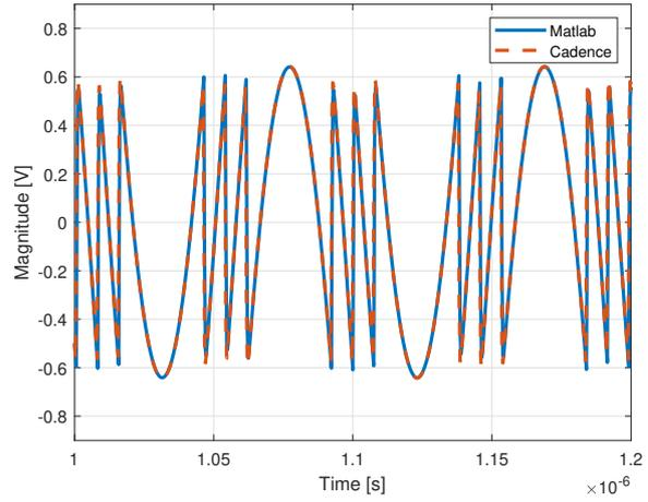
Figure 5.15: Residue signal after the gain and LPF,  $f_{in} = 11$  MHz
