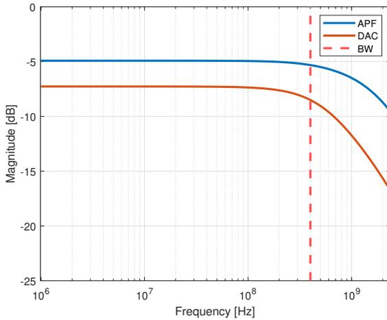
**Figure 6.12:** Magnitude response of the APF and DAC for the open loop implementation, with the LPF added
