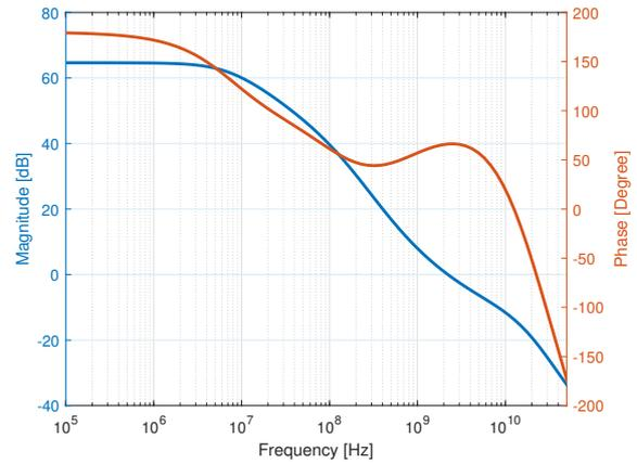
Figure 6.25: Loop gain and phase of the closed loop LPF
