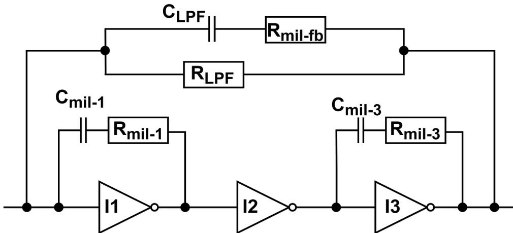
**Figure 6.23:** A single sided schematic of the closed loop LPF, the implementation of the Miller compensation
