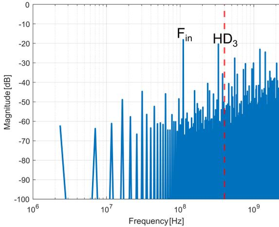
**Figure 6.2:** Spectrum of residue signal for the closed loop implementation,  $f_{in} = 110\text{MHz}$
