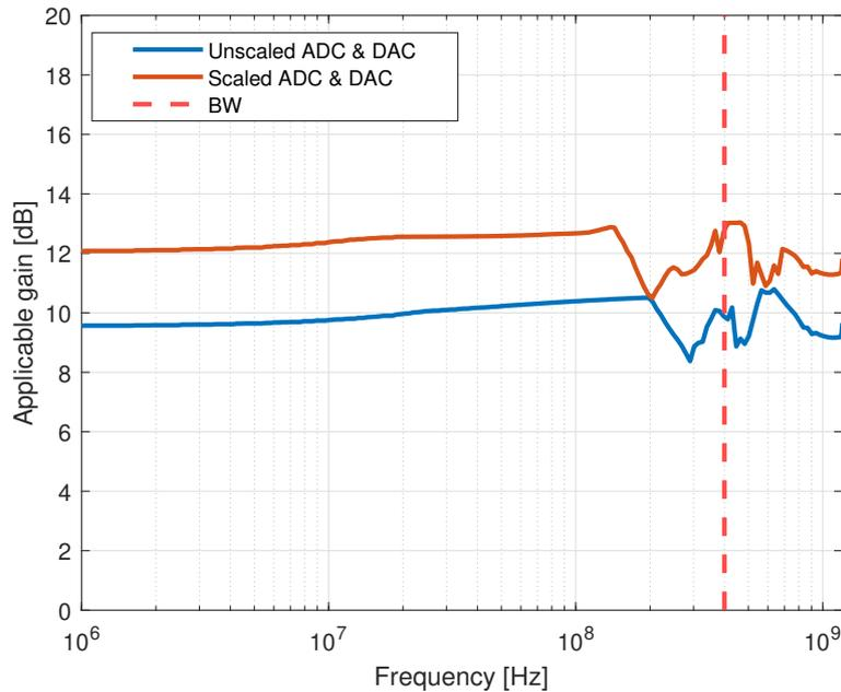
**Figure 4.24:** Gain improvement due to the scaling of the ADC & DAC
