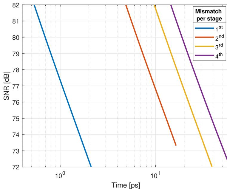
**Figure 5.7:** Time mismatch for the five-stage architecture, with 2 bit coarse ADCs
