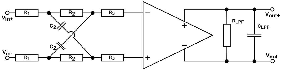
Figure 6.8: Open loop amplifier
