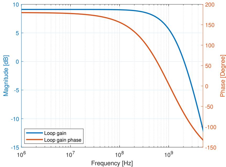
**Figure 6.20:** The open loop amplifier transfer function
