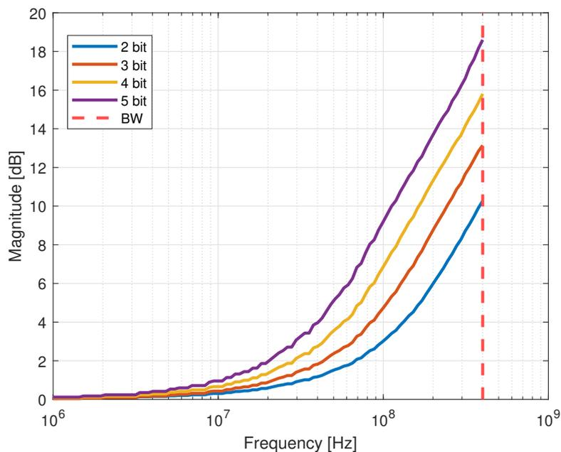
**Figure 4.13:** Gain after LPF, for different amount of bits, for an ideal latency compensation and the LPF has 3dB attenuation at 400MHz ( $f_{-3dB} = 622\text{MHz}$ ). Note that for a better visualization of the LPF impact, the DC gains are normalized to 0dB
