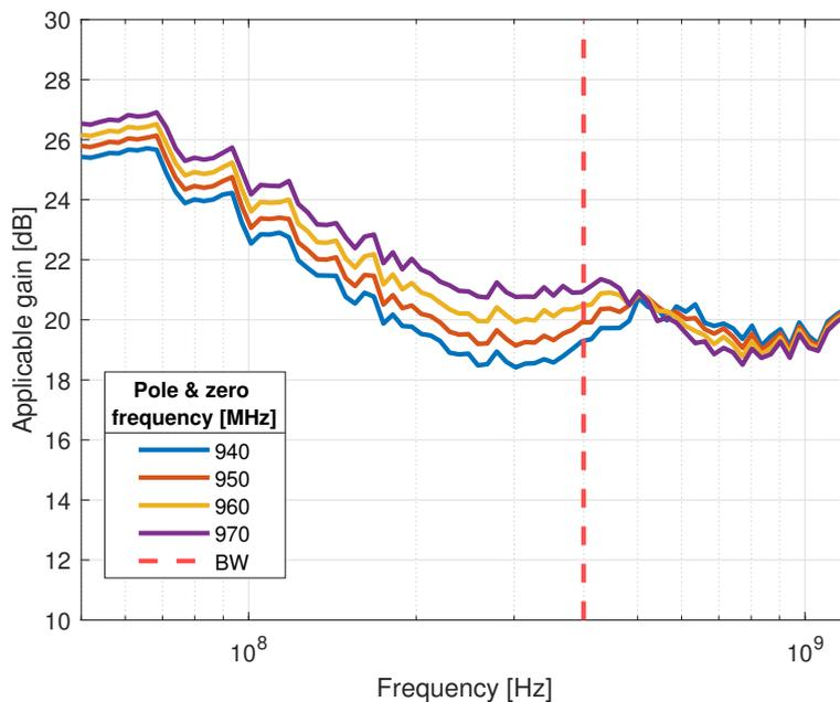
Figure 4.16: Applicable gain versus frequency, for a 4<sup>th</sup> order APF, AAF and LPF have 1.5dB attenuation at 400MHz
