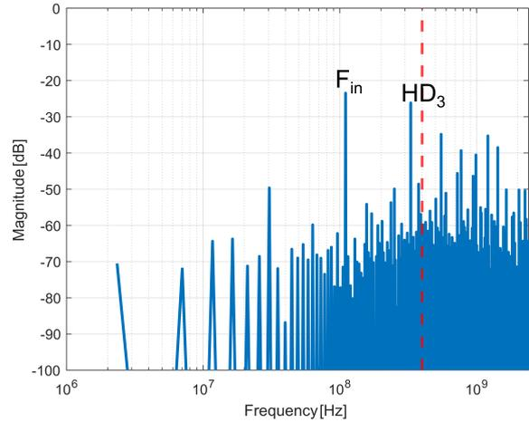
**Figure 6.3:** Spectrum of residue signal for the open loop implementation,  $f_{in} = 110\text{MHz}$
