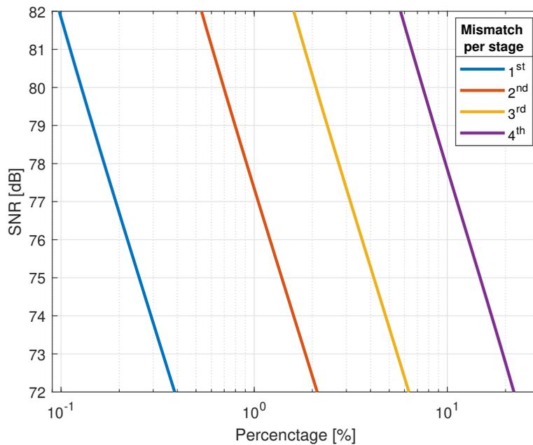
**Figure 5.5:** Gain mismatch for the five-stage architecture, with 2 bit coarse ADCs
