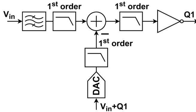
Figure 6.6: Open loop LPF implementation, 1<sup>st</sup> order in the APF, 2<sup>nd</sup> order after the inverter
