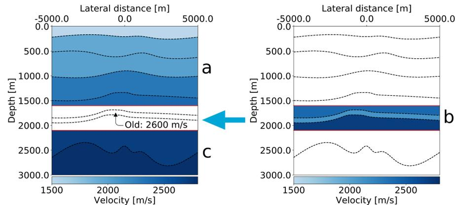
FIGURE 1 The principle of target replacement: the over- and underburden responses (a and c) are extracted from the original reflection response (left). Next, the response of the new target zone (b) is inserted (right).
