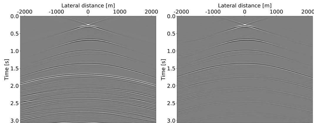
FIGURE 2 The original reflection response ( $R_C^U$ ) modeled with finite differences (left), from this the reflection response, including multiples, of unit A ( $R_A^U$ ) is extracted (right). The velocities are shown in the left of Figure 1.
