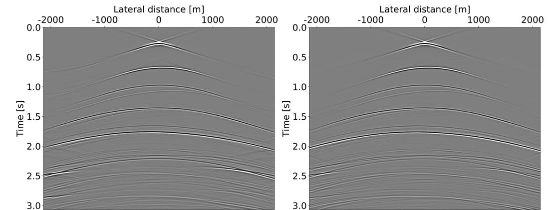
FIGURE 4 The new reflection response ( $\bar{R}_C^U$ ) retrieved with Marchenko-based target replacement (left) and reference modeled with finite differences (right). The velocities are shown in Figure 1.
