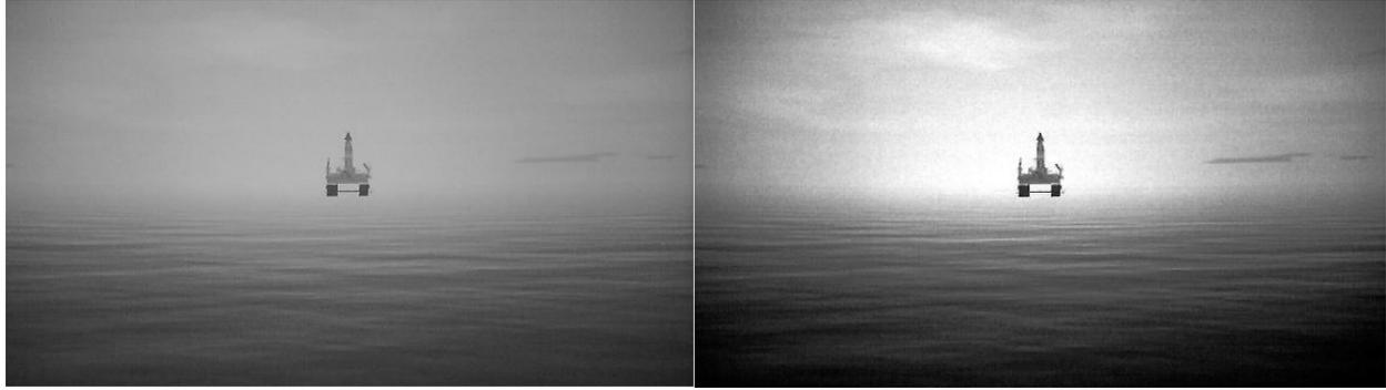
(a) Intensity image before histogram equalization. (b) Intensity image after histogram equalization.
