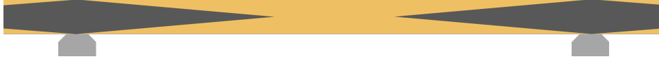
Figure 1.4: Impression of the gradual transition of timber (brown) to steel (dark grey).
