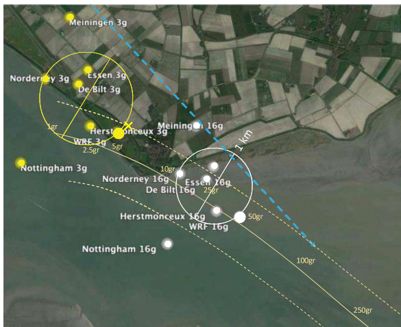
Figure 6 – Calculated impact points for the fireball of June 04, 2023, near Ellewoutsdijk, for two different sizes (16 gr -white; 3 gr – yellow) and different sounding (small dots) and model data (large dots). The circles represent an estimate of the spread in the impact point due to the slightly different weather parameters at the neighbouring weather stations or WRF model. In dashed blue, the ground projection of the trajectory is shown. Also is the impact points as carried out by GMN (Vida/Devillepoix, 2023) are also plotted (in light-yellow color).
