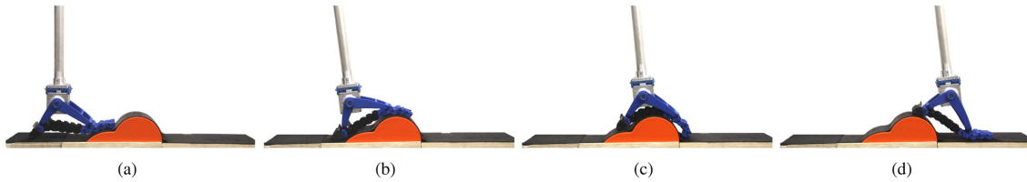
Fig. 13. Qualitative demonstration of different SoftFoot behaviors when walking on an artificial obstacle, simulating an uneven terrain: (a) initial step, where only the toes make contact with the obstacle, (b-c) stages where the entire sole is in contact, and (d) final step, where only the heel remains in contact. For this evaluation, the SoftFoot is connected to an aluminium bar and guided by an operator through the different stages of the walking.
