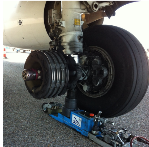
Figure 1.2: Example brake assembly of an 737NG main landing gear [3]
