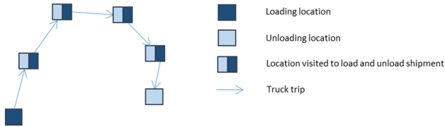
Figure 5.6. A hypothetical example of a tour sequence constructed with the second tour sequence algorithm. We visit alternately loading and unloading locations, and visit remaining unloading locations afterwards.
