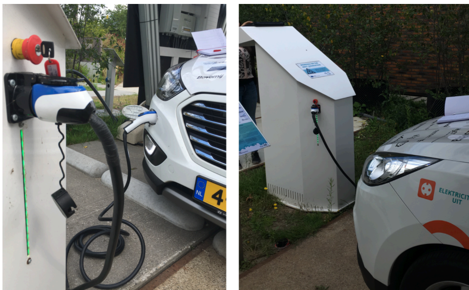
Figure 3.2: Experimental setup of the FCEV operating in V2G mode.
