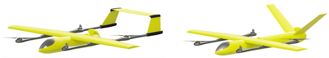
Figure 7.1: Left: Twin boom configuration, Right: Quadplane configuration [40]
