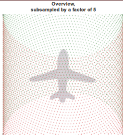
Figure 3.1: RIEGL VQ-840-GE elliptical LIDAR scan pattern[8].
