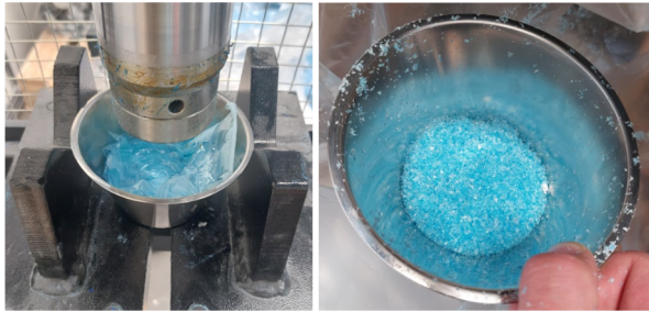
Fig. 15. Left; Compressing of ALP, Right; Shredded ALP
