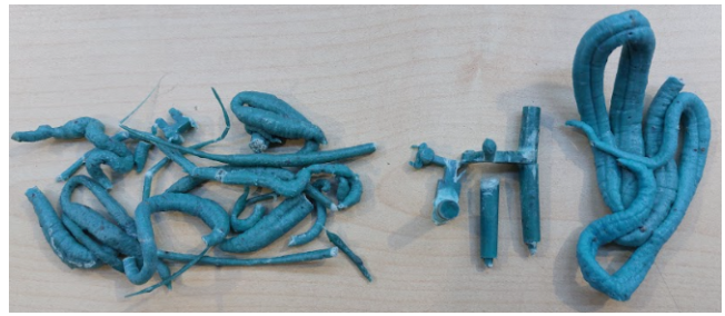
Fig. 16. ALP melted manually in the Babyplast injection molding machine
