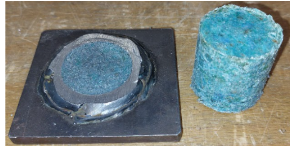
Fig. 17. Recycled plastic using high-pressure molding setup 1
