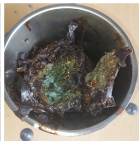
Fig. 24. Images taken from the different melting trial (First picture of Trial 6 - ALP after 50 min in an oven at 250 degrees Celcius. Second picture of Trial 6 - Partially melted ALP after 50 min in an oven at 300 degrees Celcius.)
