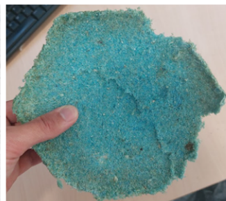
Fig. 24. Images taken from the different melting trial (First picture of Trial 6 - ALP after 50 min in an oven at 250 degrees Celcius. Second picture of Trial 6 - Partially melted ALP after 50 min in an oven at 300 degrees Celcius.)
