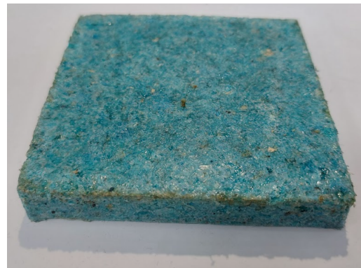
Fig. 21. Recycled ALP using the spring high-pressure molding setup
