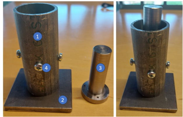
Fig. 6. First high-pressure melting setup: 1. Steel Pipe, 2. Closure Plate Welded to Steel Pipe, 3. Compressing Rod, 4. Bolts Ensuring Compressing Rod Locking.
