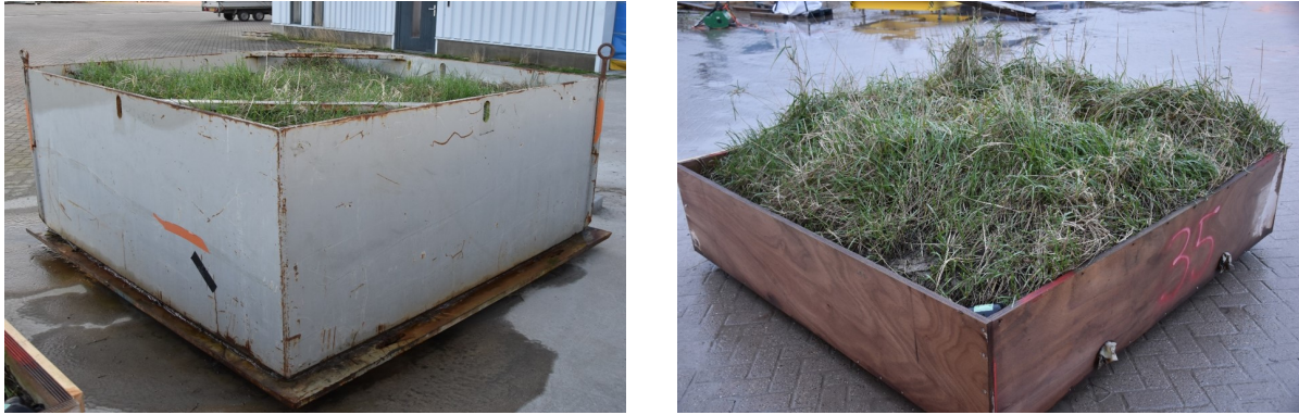
Figure 3.4: Salt marsh blocks. a) Steel block of dimensions 2.0x2.0x0.7 m, b) Wooden block of dimensions 2.2x2.2x0.4 m
