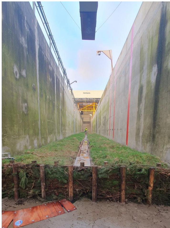
Figure 3.5: Salt Marsh blocks located in the flume with a brushwood dam on the cliff
