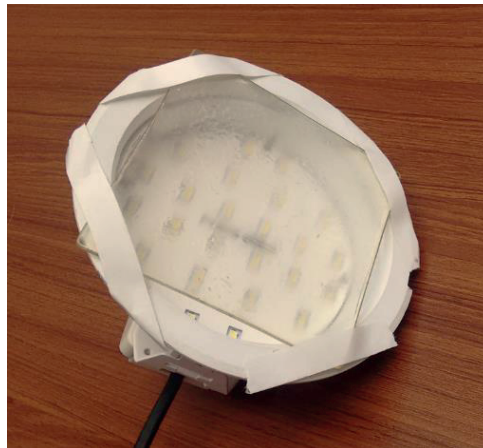
Figure 2 PMMA specimen mounted on the luminaire for integrating sphere measurement
