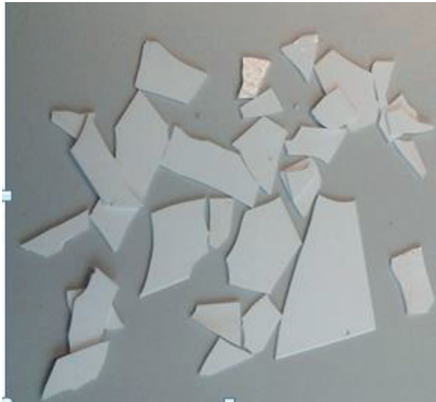
Figure 6 Specimen smashed after 4000 hours of humidity test during handling
