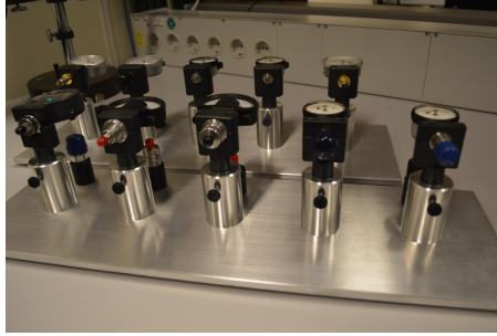
Figure 3.25: Coaxial connector gauges used for measurement of pin gap at VSL.
