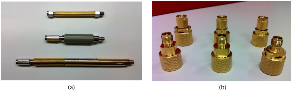
Figure 2.19: (a) Metrology grade coaxial air-dielectric transmission line standards. (b) An overview of metrology grade coaxial SOLT calibration kit.
