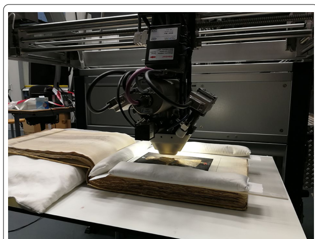
Fig. 6 View of the MA-XRF analytical setup used for the scrapbook. © Leila Sauvage, Rijksmuseum
