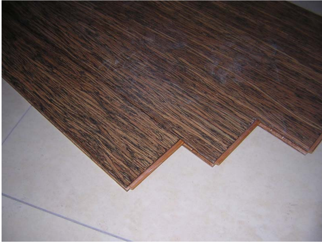
Figure 2: An example of flooring panels based on the Strand Woven Bamboo technique
