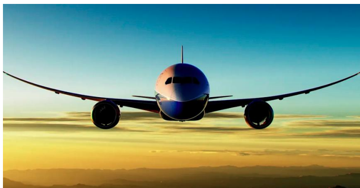
Figure 1.3: Wing Flex of a Boeing 787 inflight
