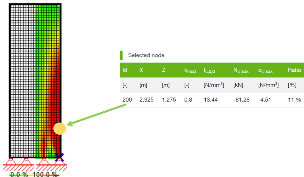
Figure E.13 – Compressive stresses as determined in calculatis
