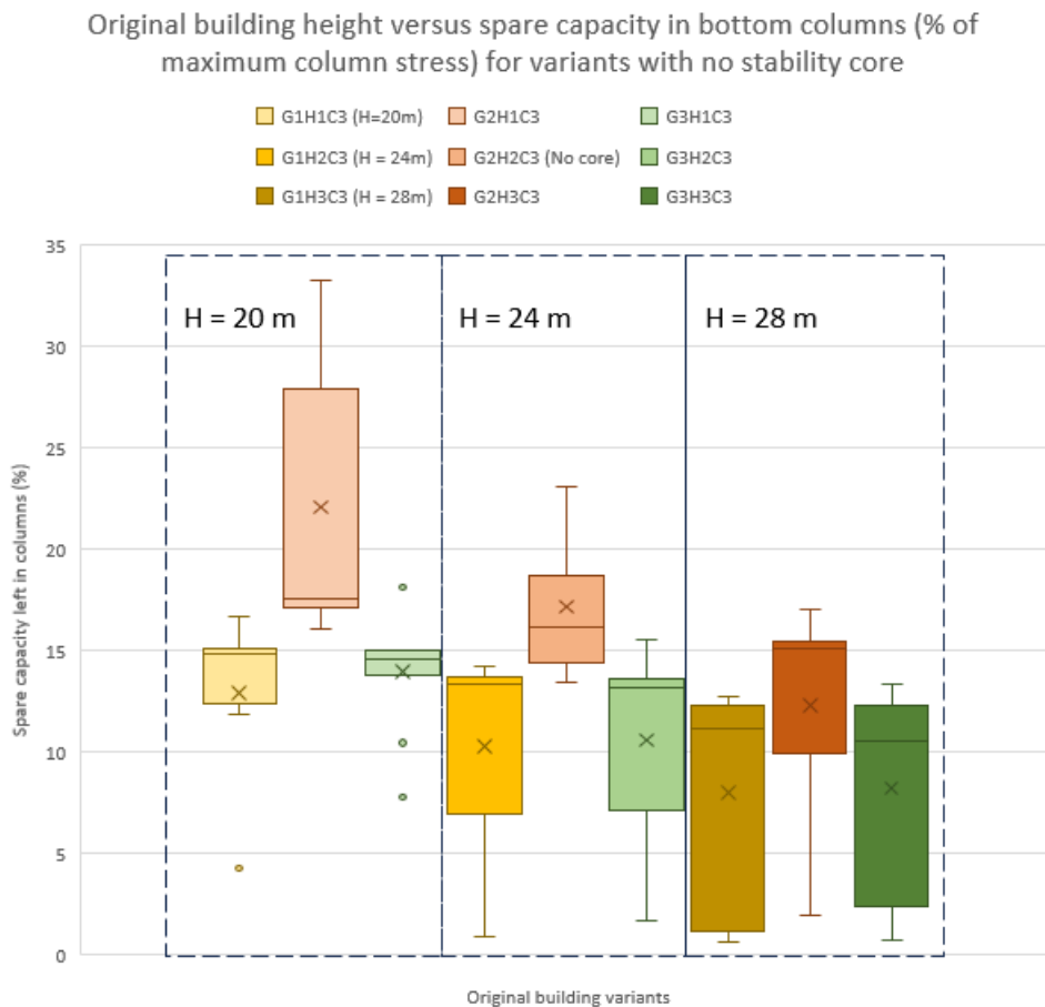
Figure 7.9 Height of the original structure vs. spare capacity left in the bottom columns (%) for variants with no stability core
