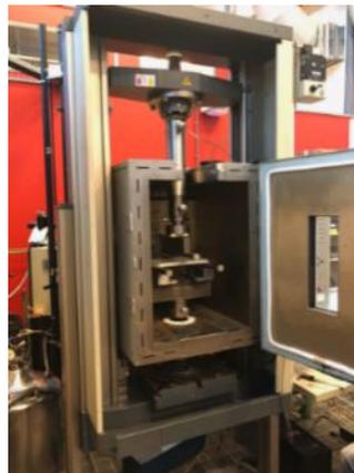
Fig. 11 3-Point bending test setup for elevated temperatures.
