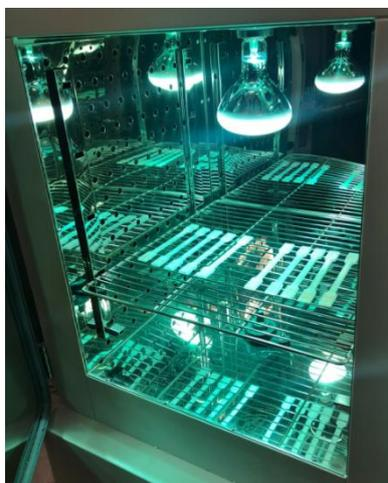
Fig. 3 Accelerated UV source with 3D printed specimens.
