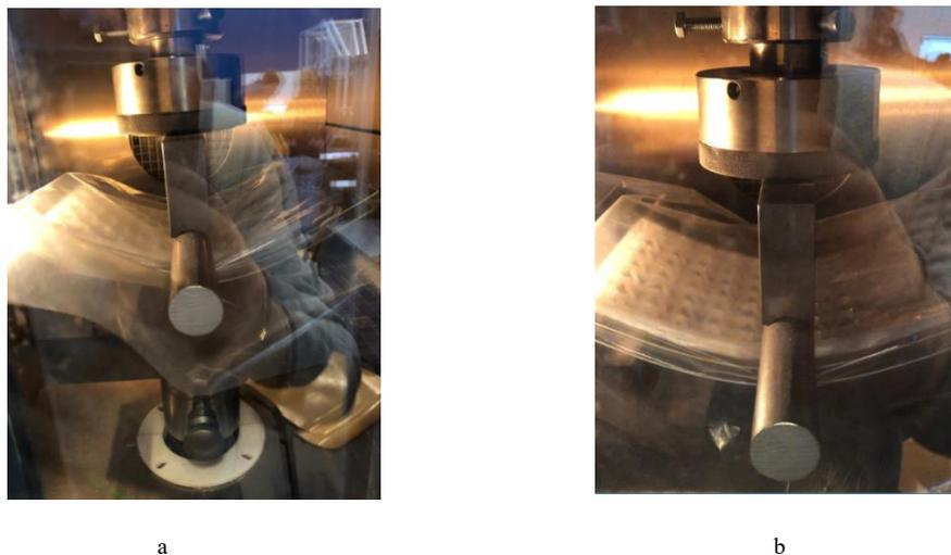
Fig. 13a) Composite panel (honeycomb core) with a deflection of 50mm at 80 °C, b) Composite panel (truss core) with a deflection of 50mm at 80 °C.
