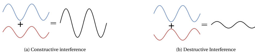
Figure 3.4: Interference of two waves of amplitude A and B are shown. In constructive interference as they are in phase the final wave has an amplitude of A+B . In the case of destructive interference the waves are out of phase by 90^\circ giving an amplitude of A-B for the final wave.
