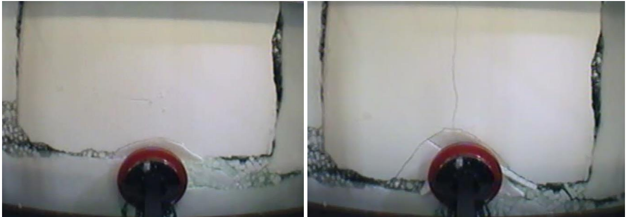
Figure 6. Image from model test video. Encounter between the structure and a large ice floe of 165x165m (HSVA 2010b)
