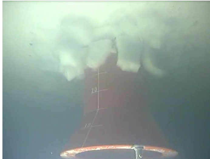
Figure 12. Ice rubble accumulates near the structure, beneath the ice, still from model test video (HSVA 2010a)
