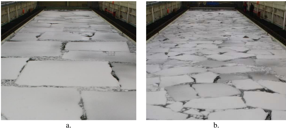
Figure 4. Overview of the floe distribution in the ice basin a) large floes and b) smaller floes (HSVA 2010a)
