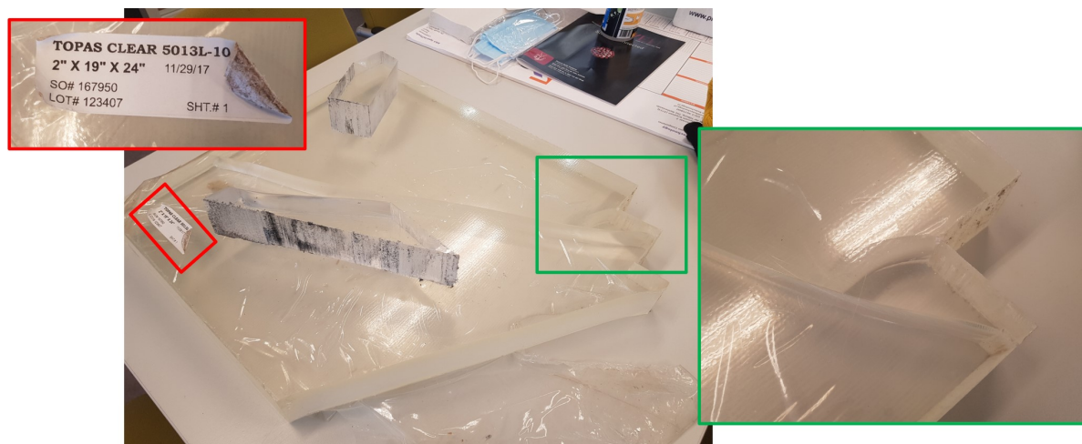
Figure 2.10: Several photos of a 2x19x24 inch 5013-L TOPAS sheet used for fabricating sub-millimeter optical components. Smaller pieces were cut from the corner. Over time during idle storage cracks appeared. The red zoomed section shows the sheet label with product information. The green zoomed section shows the corner where smaller pieces were cut from.
