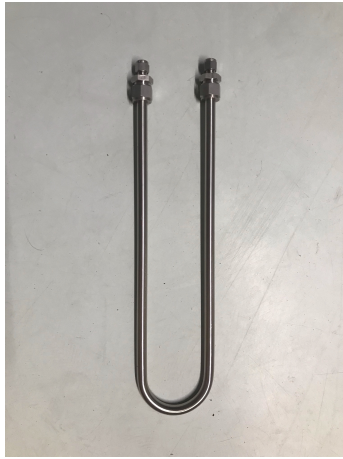
(a) Configuration B: 62.8 cm 3 inside volume
