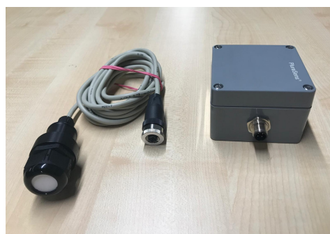
Figure 3.2: Evikon sensor probe with sensor transmitter
