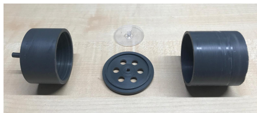
(b) PVC sensor housing including umbrella valve
