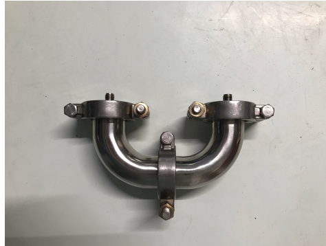
(b) Configuration C: 230.9 cm 3 inside volume
