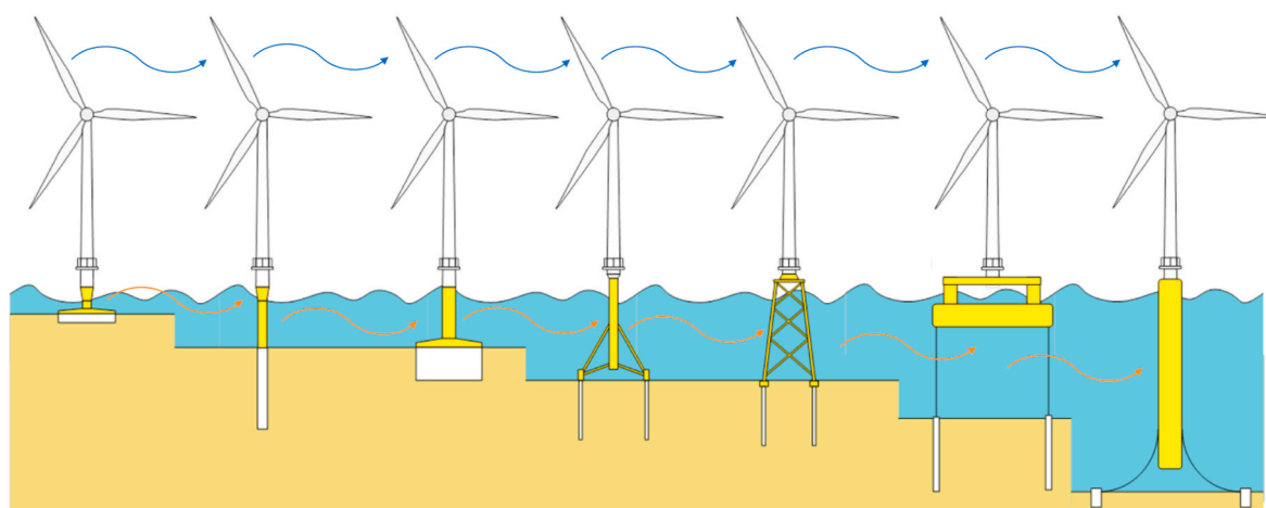
Fig. 13. Typical support structures of offshore wind turbines [132].
