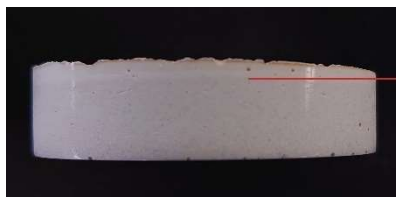
Figure 4.2.8 Lateral view of GP mortar sample before heat treatment. Segregation is indicated by the red line.
