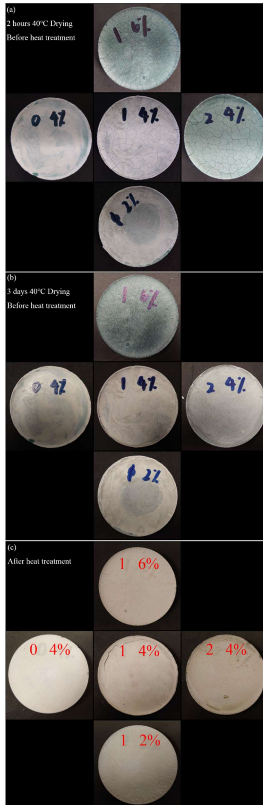
Figure 4.2.5 AAS Samples condition after: (a) drying for 2 hours at 40°C; (b) drying until relative stable mass (~3 days) at 40°C; and (c) heat treatment. Samples were marked with two values: the first one indicates the M_s of the mixture; the second one in percentage indicates the alkali content
