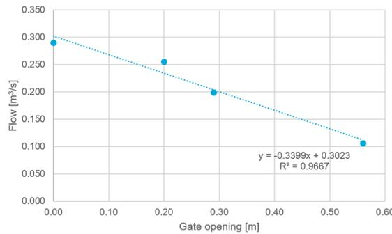
Figure 15.5: Relation between the discharge in side channel and the opening of the gate at the first bifurcation. Discharge before bifurcation is  $0.534 \text{ m}^3/\text{s}$ .
