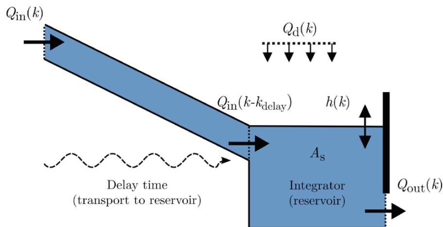
Figure 15.1: Integrator Delay model of a single canal reach [65].
