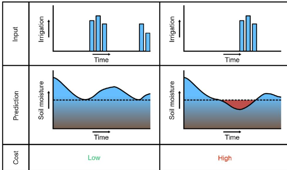
Figure 15.6: Visualisation of the objective function.
