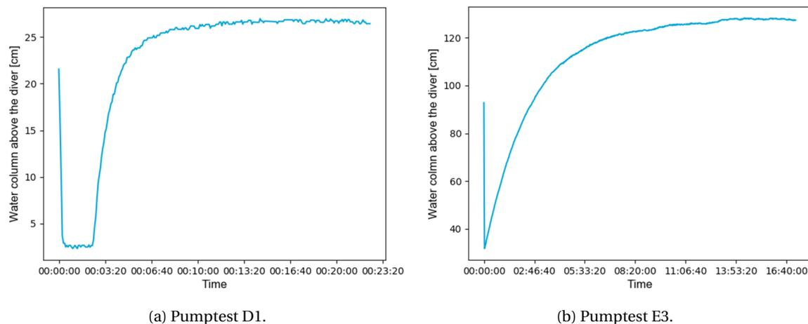
Figure B.3: Diver data showing the head difference over time during the slug test.
