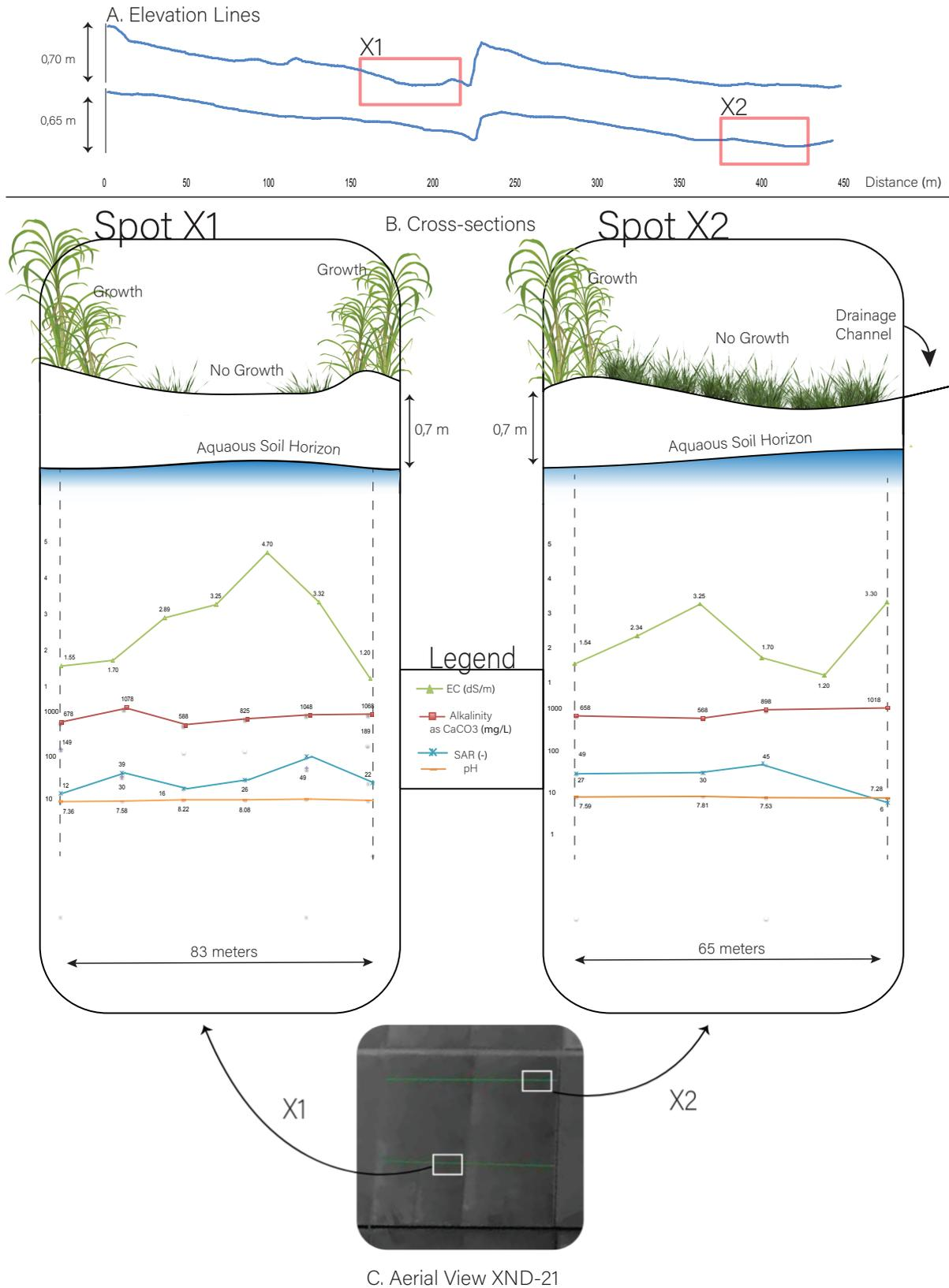
Figure 10.7: Visualisation of bad spots X1 and X2, showing the EC, sodium adsorption ratio, pH and alkalinity concentration of the groundwater.
