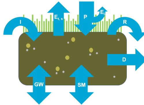
Figure C.1: Schematic overview water balance
