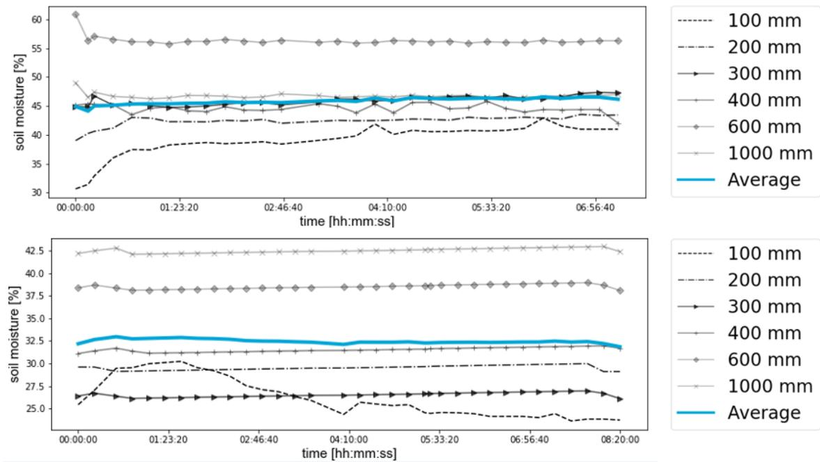
Figure E.2: Infiltration test results in XND-21 (up) and XNE-21 (down).
