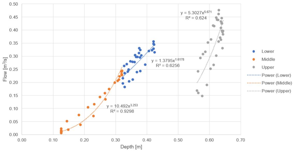
Figure D.2: Rating curves for three locations.
