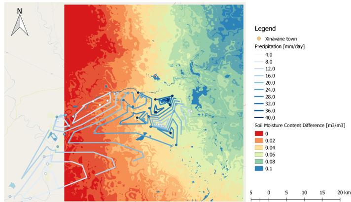
Figure 16.12: Spatial distribution of the SMC difference between for and after the rain event of 14 April 2017.
