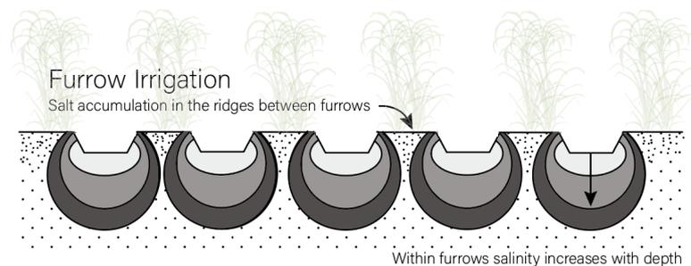
Figure 8.2: Locations of salt accumulation within the soil when furrow irrigation is applied and salts are not adequately leached. Salts will accumulate on the ridges between furrows as this is where the water is pulled towards by the roots of the sugarcane. Underneath the furrows salts will increase the deeper you go: The darker the color of the ring, the higher the salt concentration.
