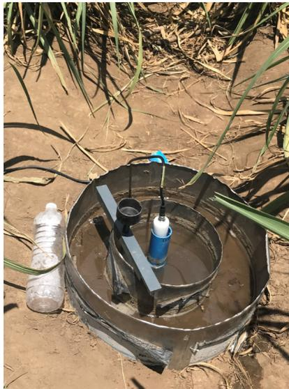
Figure E.1: Infiltrometer.
