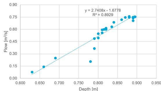
Figure 15.4: Rating curve of the main weir.
