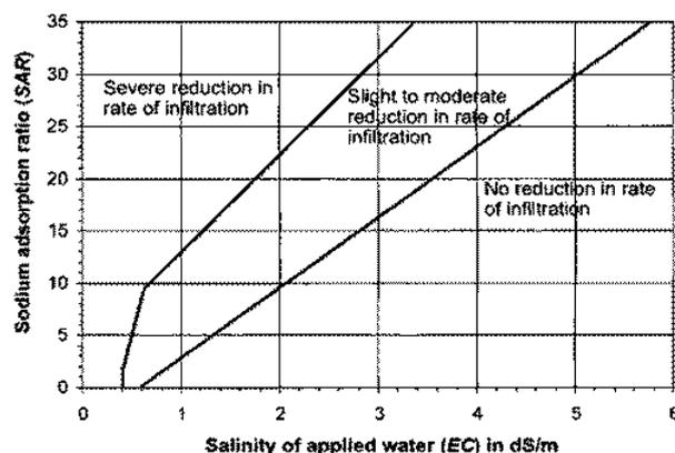
Figure 8.3: Infiltration risk assessment. As can be seen in the figure, there can be benefits of high saline water in heavy soils where the infiltration is low. The sodium adsorption ratio (explained in the 'Sodicity' section) also plays an important role in determining the infiltration reduction through its affect on the soil. [37]
