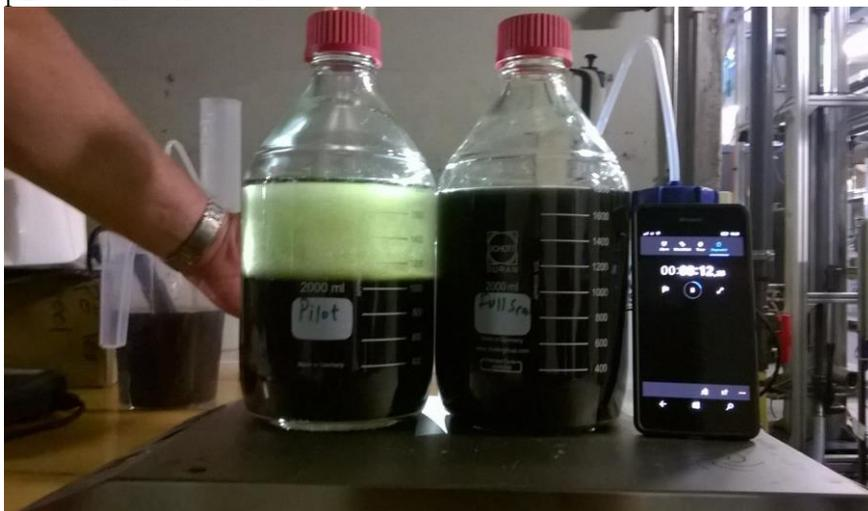
Figure 26: Secondary backwash experiment T = 8 min, left contains backwash water from the pilot filter while applying AOCF, right jar is backwash water originating from a RSF in Katwijk
