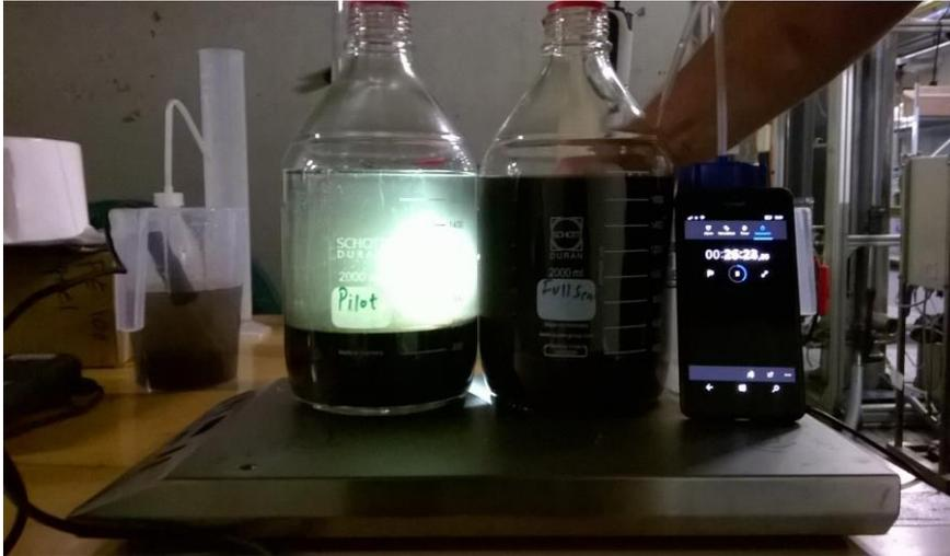
Figure 27: Secondary backwash experiment  $T = 26$  min, left contains backwash water from the pilot filter while applying AOCF, right jar is backwash water originating from a RSF in Katwijk
