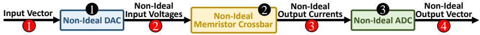
Figure 3.4: An overview of the VMM Model Generator's second approach: using analytical models.
