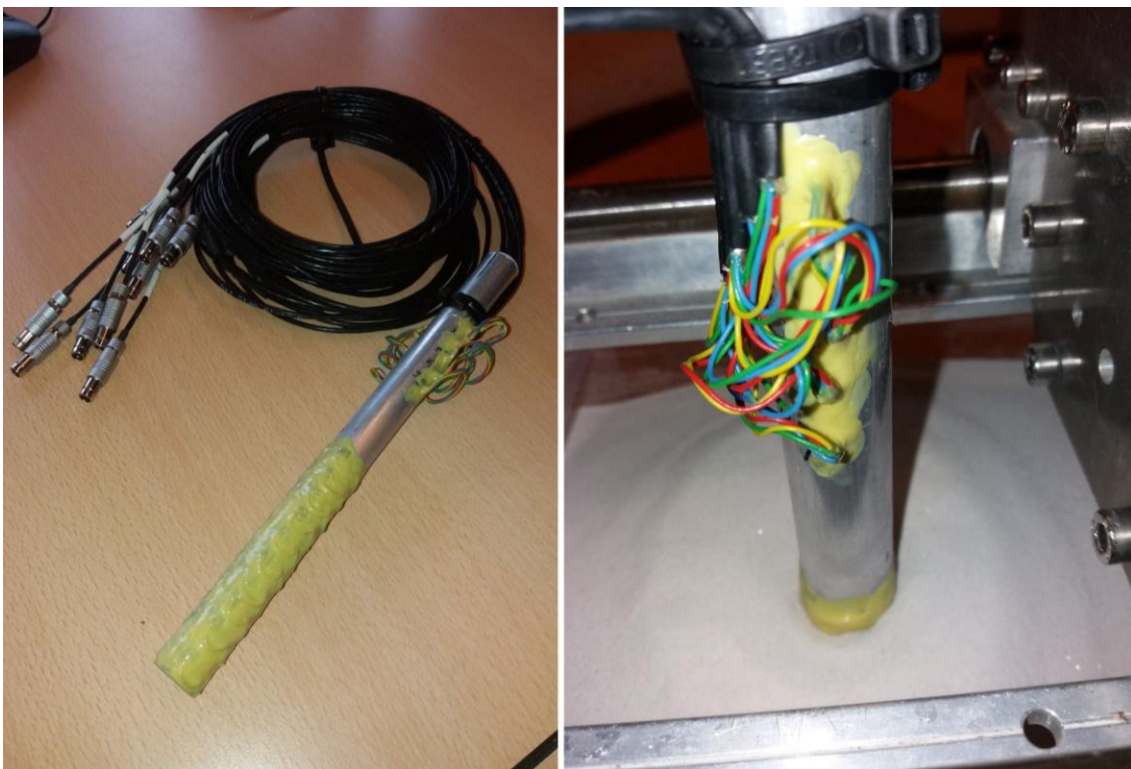
Appendix Figure 2 Pile used for the centrifuge experiment in and out the sample.
