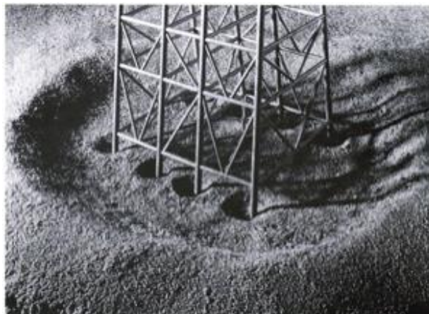
Figure 1.1 Local scour is observed in the hole that has been formed in each pile, while the global scour can be observed around the whole pile structure. Whitehouse, 1997
