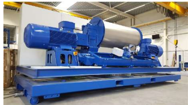
Figure 11.2: Winch produced by Dromec for Kitepower systems ground station 2
