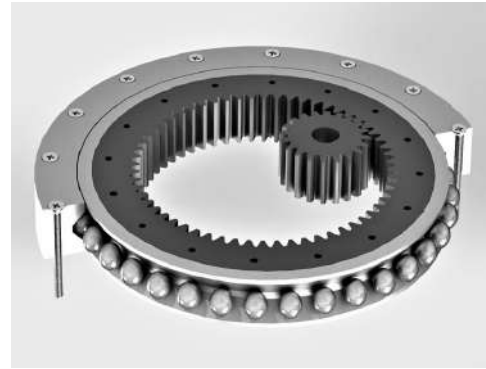
Figure 7.7: Internal gear slew bearing. In this image, the inner slew bearing ring rotates, while the outer is stationary and holds the structure. The small gear represents the motor rotating the inner ring.
