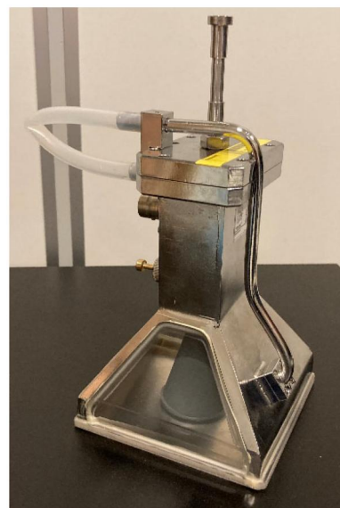
Figure 2. Lucite cone applicator (LCA). The antenna operates at 434 MHz and has an aperture of 10 \times 10 \text{ cm}^2 .
