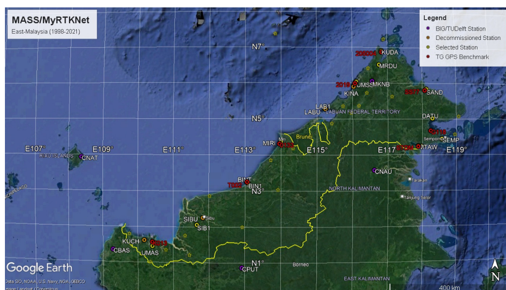
Figure 7. Location of 17 MASS/MyRTKNet and 1 GEODYSSSEA stations at 12 locations (of which 9 are near the tide gauges) in East Malaysia. Shown also are the 8 tide-gauge benchmarks (in red). Additionally, the 20+ other MyRTKNet stations (including 3 off-shore) currently operated by
