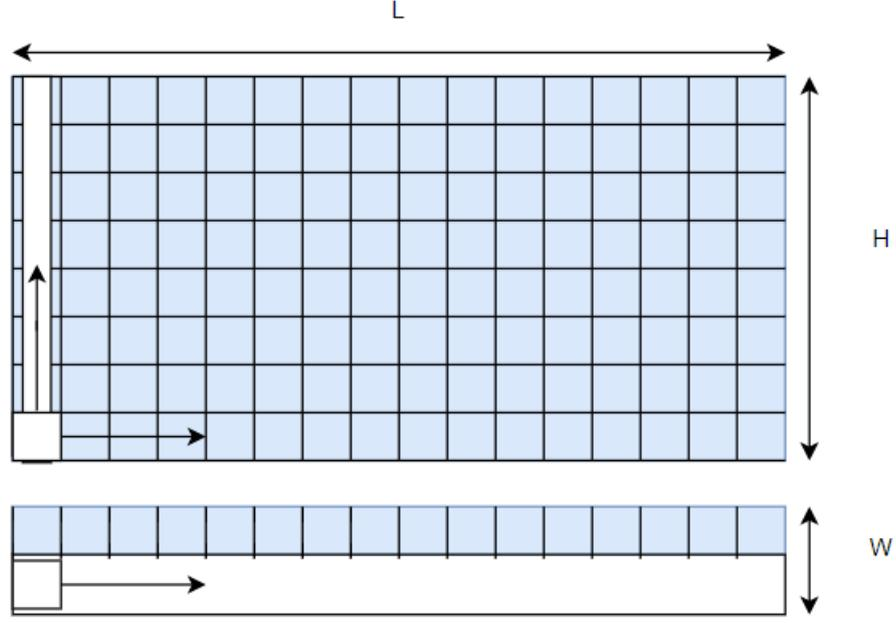
Figure 9: Schematic of a Miniload AS/RS with a side-view (top) and a birds-eye view (bottom)
