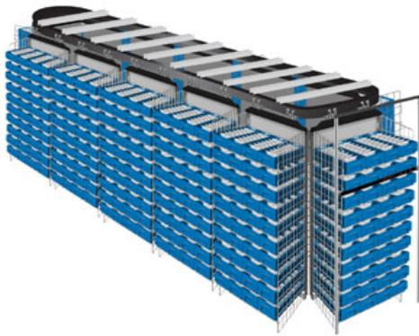
Figure 6: Vertical lift module (Retrieved from [mhi.org](http://mhi.org))
