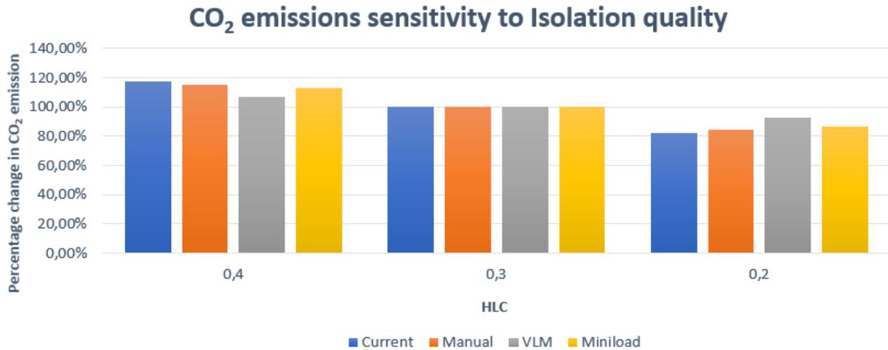
Figure 17: CO<sub>2</sub> emission sensitivity to isolation quality for each configuration
