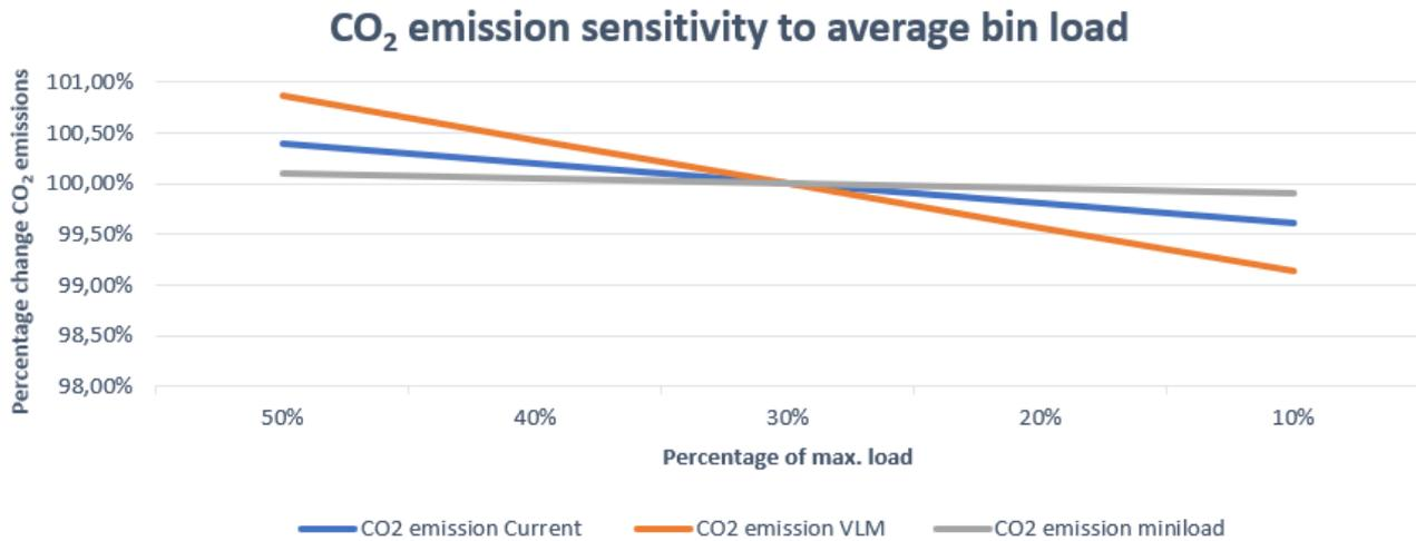
Figure 15: CO<sub>2</sub> emission sensitivity to average bin load for each configuration
