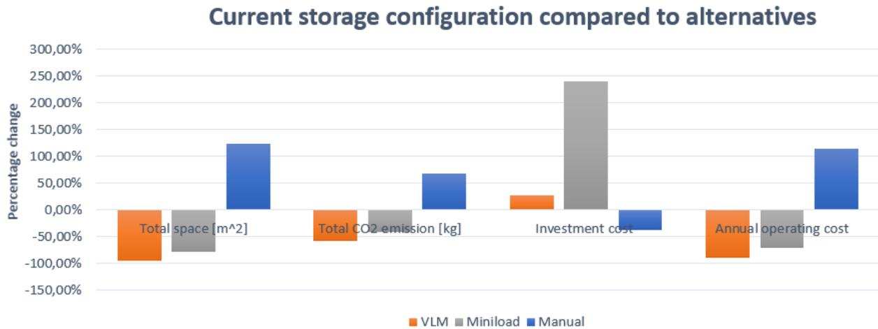
Figure 1: Comparison of current storage configuration and the considered alternatives
