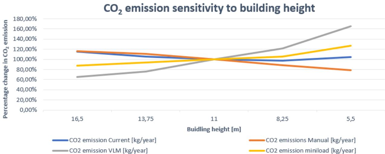
Figure 12: CO<sub>2</sub> emission sensitivity to warehouse height for each configuration
